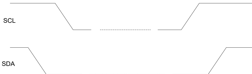
Figure 9. I 2 C START and STOP Condition Timing
