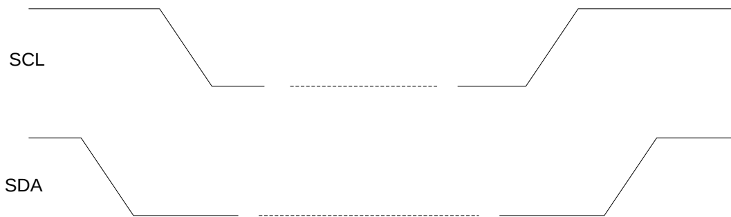
Figure 16. I 2 C START and STOP Condition Timing
