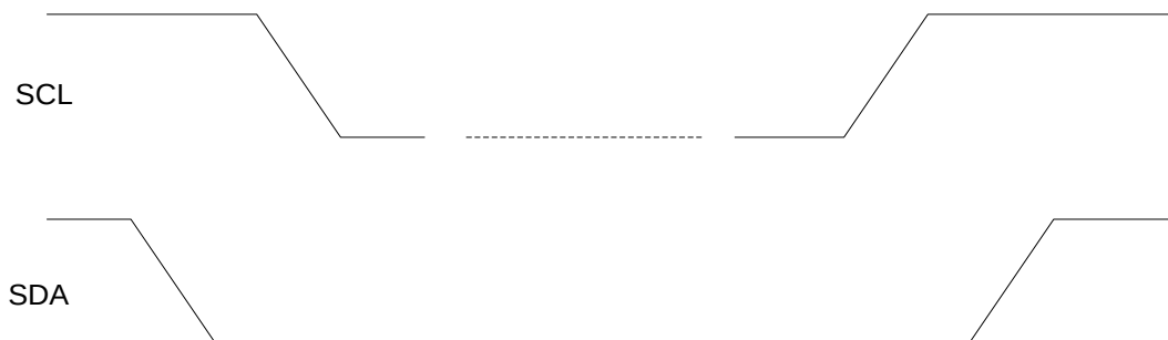
Figure 11. I 2 C START and STOP Condition Timing
