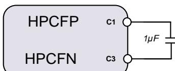
Figure 42. Charge pump flying capacitor
