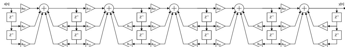
Figure 22. Cascade of five biquad filter stages
