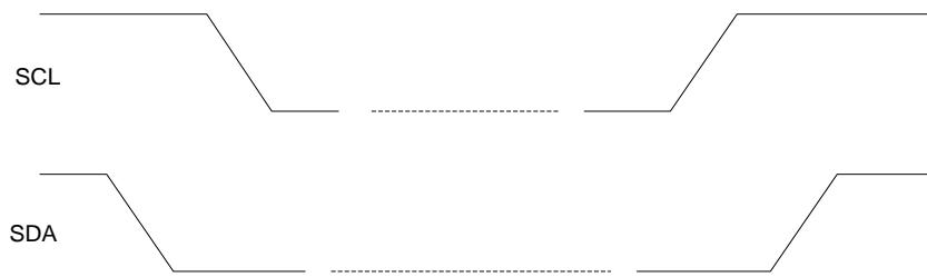
**Figure 26. Timing of I<sup>2</sup>C START and STOP conditions**
