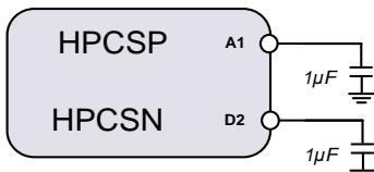
Figure 41. Charge pump decoupling
