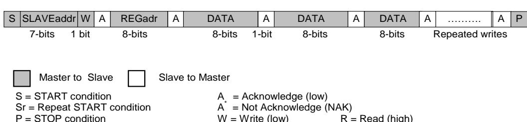
An alternative Repeated-write mode that uses non-consecutive slave register addresses is available using the [cif\\_i2c\\_write\\_mode](#) register. In this Repeat mode ([cif\\_i2c\\_write\\_mode](#) = 1), the slave can be configured to support a host's repeated write operations into several non-consecutive registers. Data is stored at the previously received register address. If a new START or STOP condition occurs within a message, the bus returns to IDLE mode. This is shown in [Figure 31](#).
