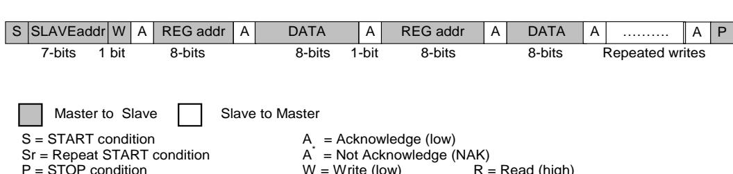
In Page mode ([cif\\_i2c\\_write\\_mode](#) = 0), both Page mode reads and writes using auto incremented addresses, and Repeat mode reads and writes using non auto-incremented addresses, are supported. In Repeat mode ([cif\\_i2c\\_write\\_mode](#) = 1), however, only Repeat mode reads and writes are supported.
