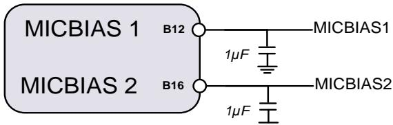
Figure 39. MICBIAS decoupling
