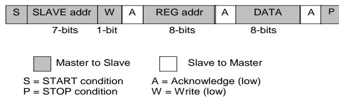
**Figure 27. I<sup>2</sup>C byte write (SDA signal)**
