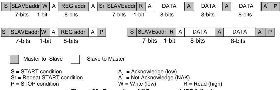
The slave address after the Repeated START condition must be the same as the previous slave address.
