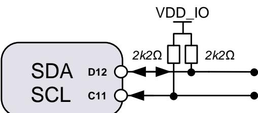
Figure 43. I<sup>2</sup>C pull ups
