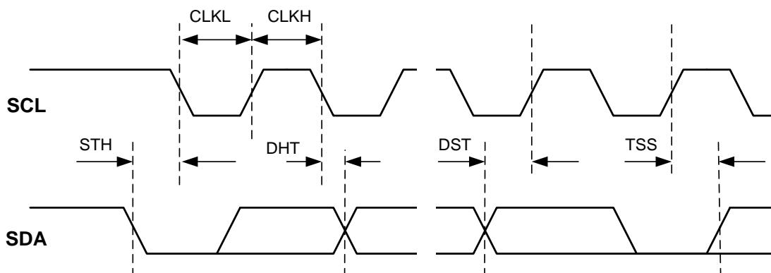
Figure 5. I<sup>2</sup>C bus timing
