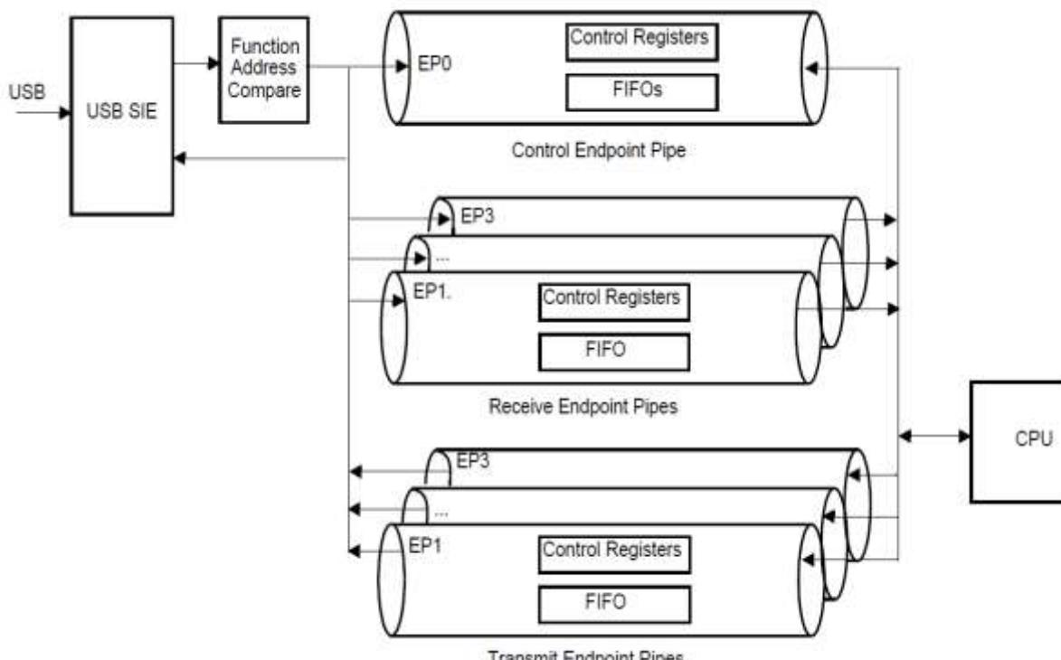
**Figure 96. Endpoint operation**
