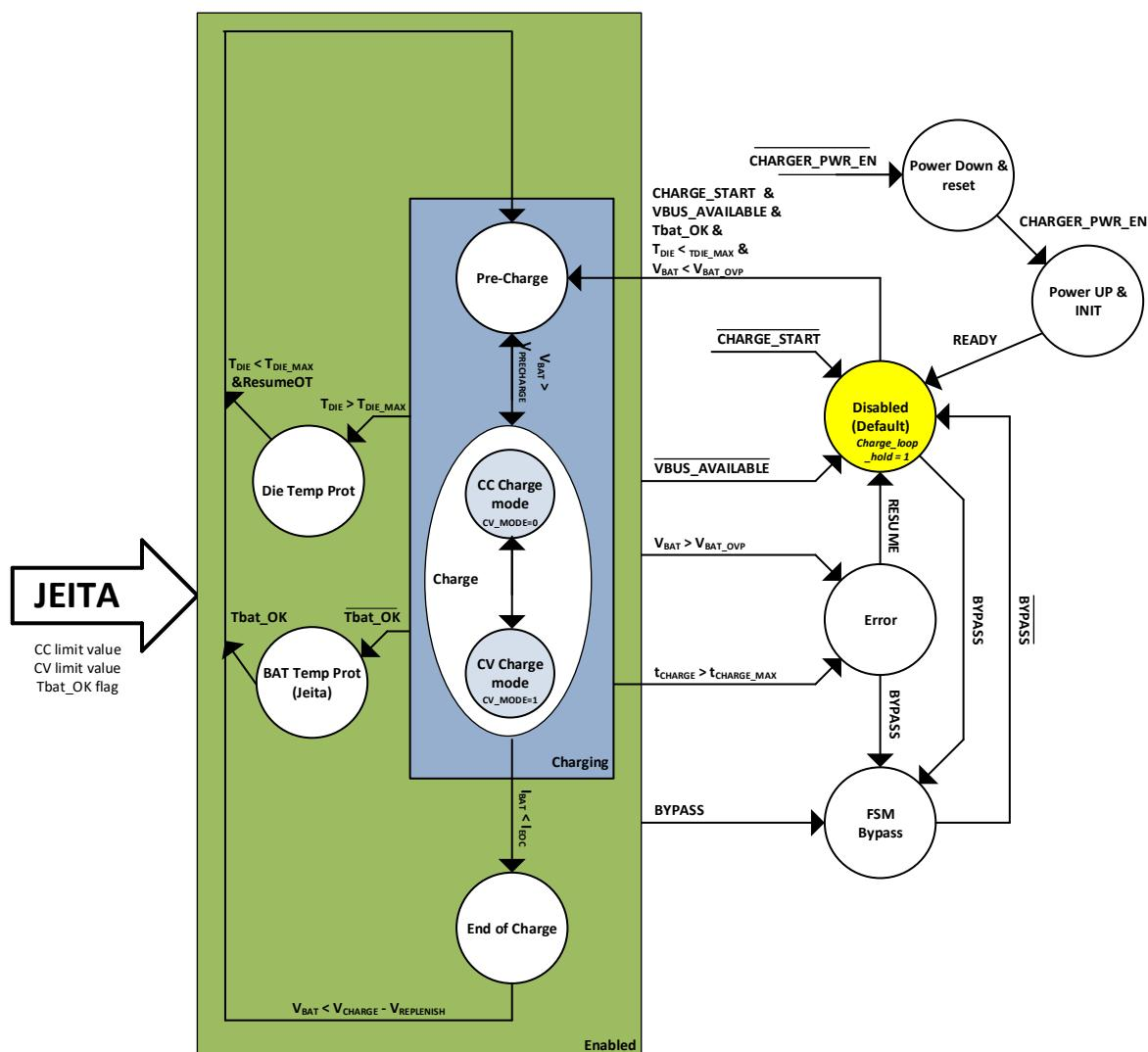
Figure 18. Charger hardware finite state machine diagram
