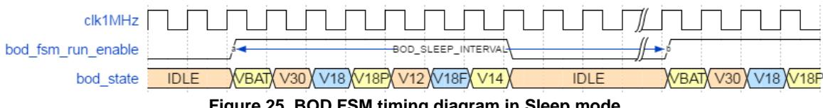
Figure 25. BOD FSM timing diagram in Sleep mode
