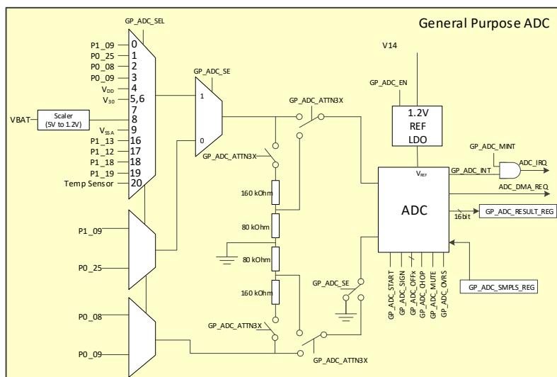
Figure 60io General-purpose ADC block diagram
