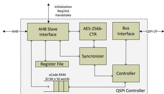
Figure 40. QSPIC flash controller block diagram
