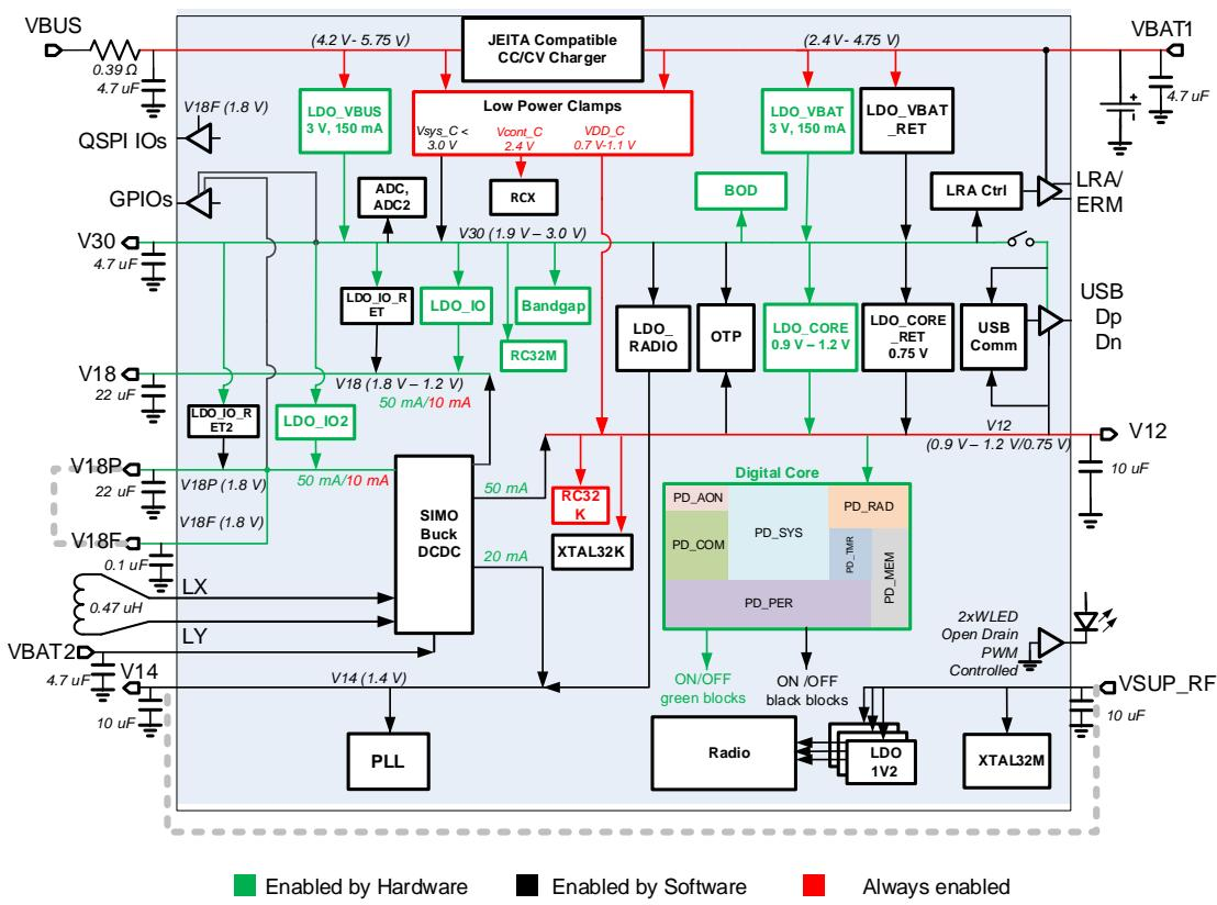
[Figure 15. Power management unit architecture](#)
