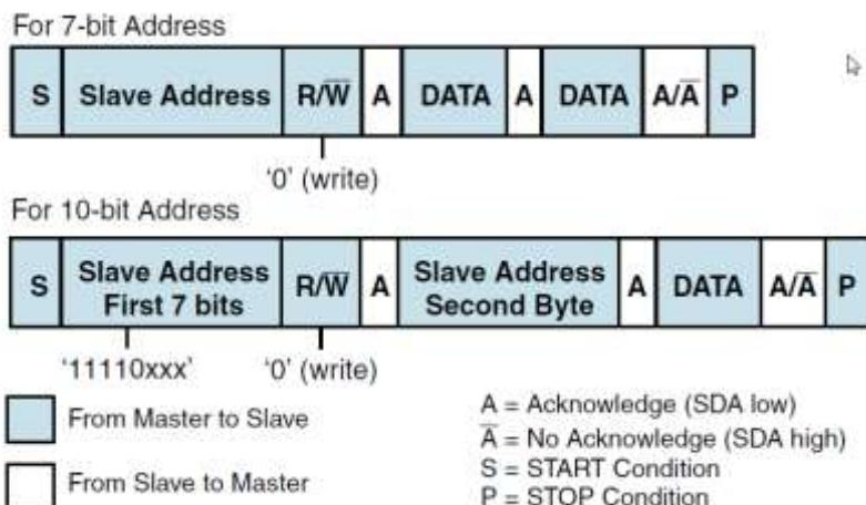
**Figure 75. Master-Transmitter protocol**
