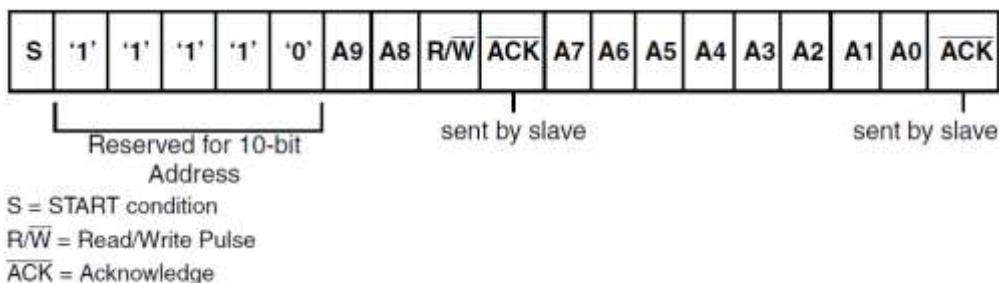
Figure 74. 10-bit address format
