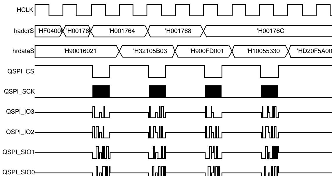
Figure 46. QSPI Split burst timing for low power (QSPI\_FORNSEQ\_EN=1)
