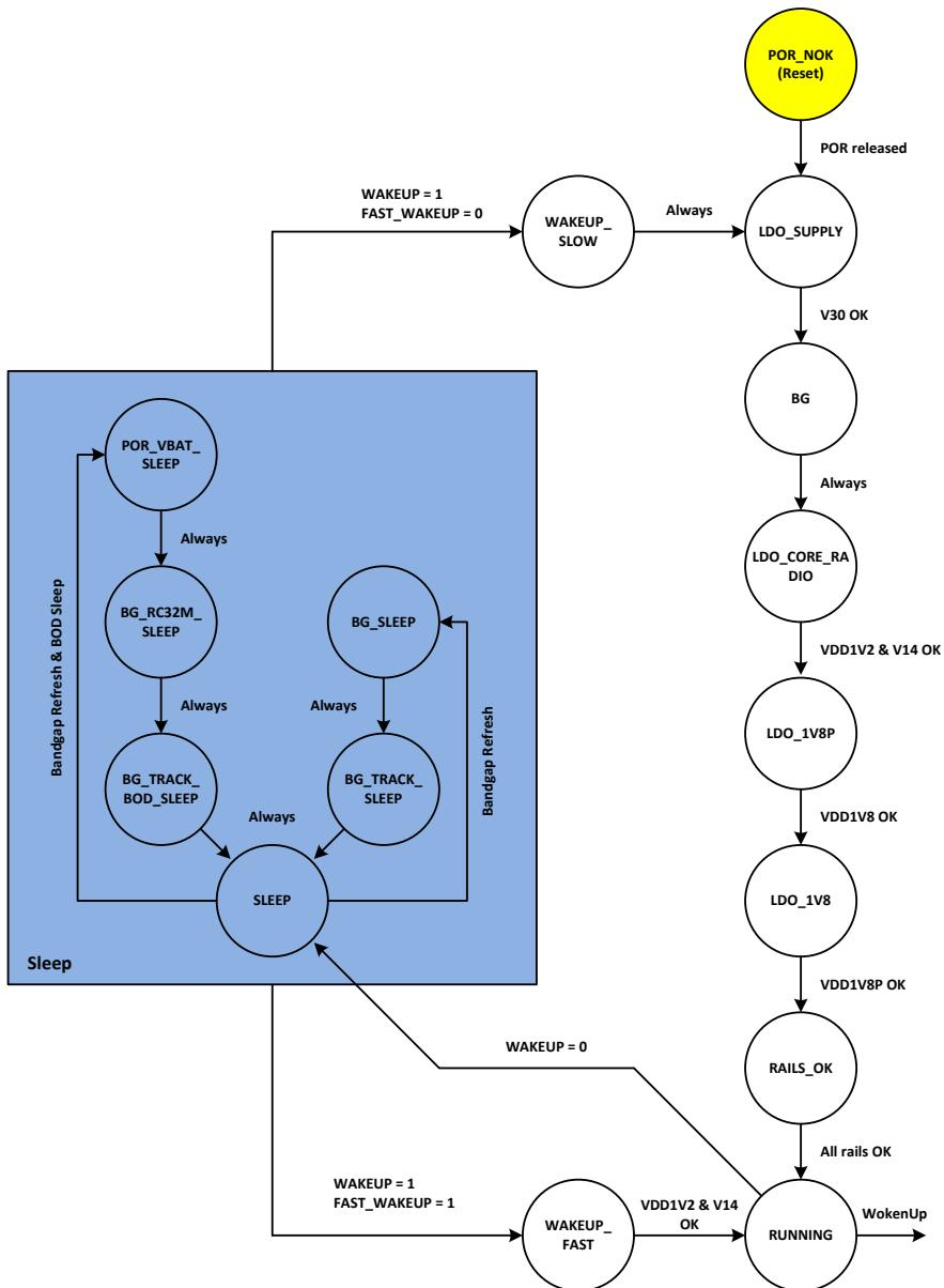
**Figure 8. POWERUP, WAKEUP, GOTO Sleep hardware FSM**
