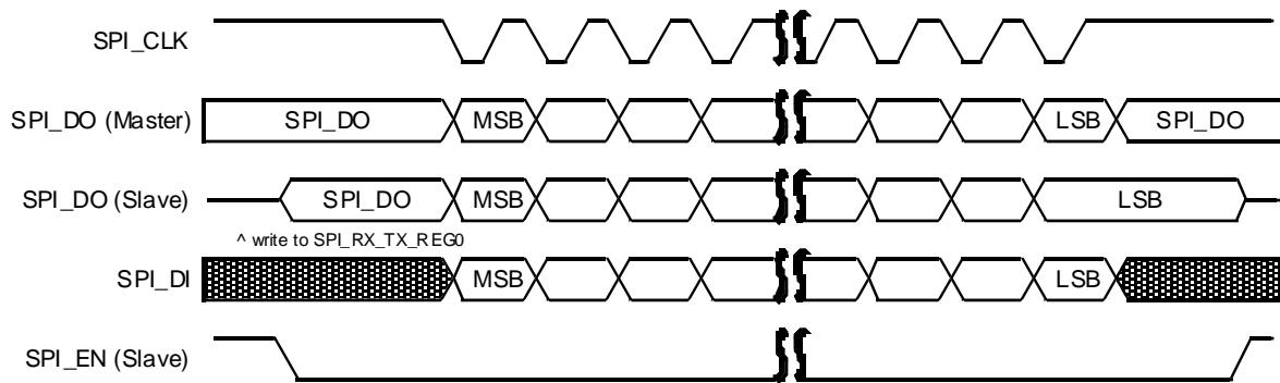
Figure 90. SPI Master/slave mode 3: SPI\_POL=1 and SPI\_PHA=1
