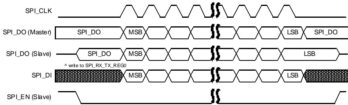
Figure 88. SPI Master/Slave mode 1: SPI\_POL=0 and SPI\_PHA=1
