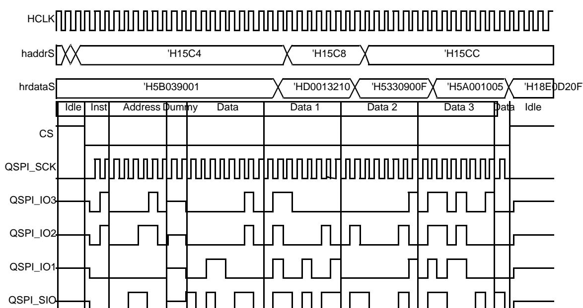
Figure 47. QSPI Burst timing for high performance (QSPI\_FORNSEQ\_EN=0)
