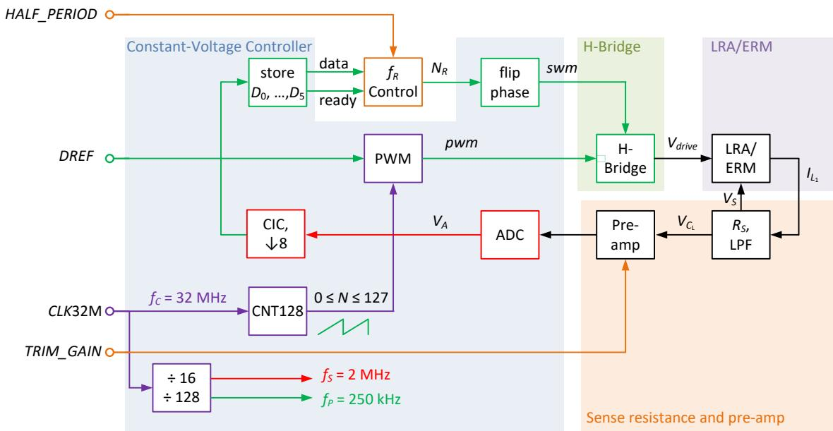
Figure 105. Block diagram of the haptic driver
