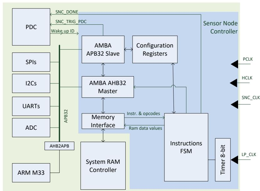
Figure 33. Sensor node controller block diagram
