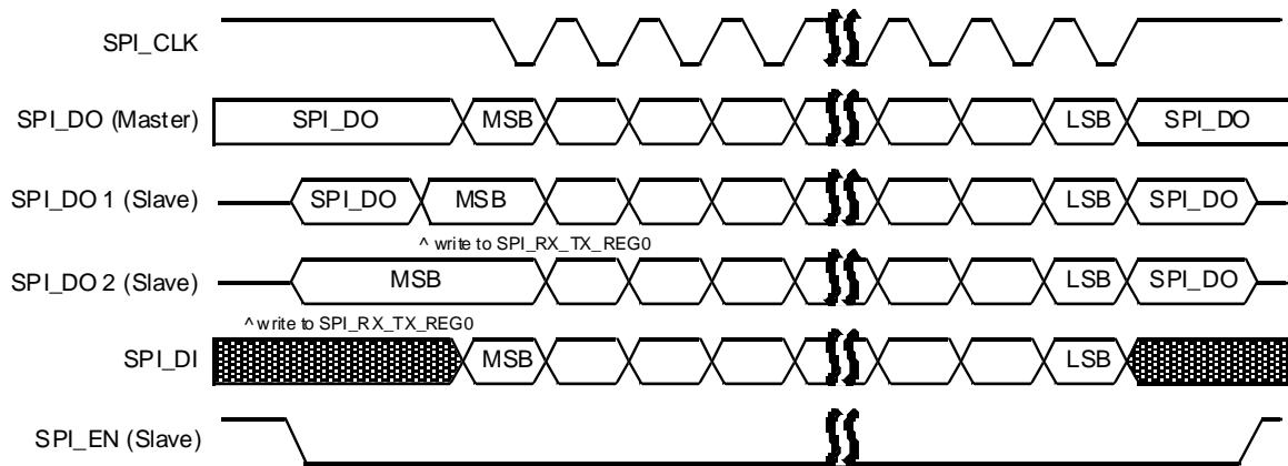
Figure 89. SPI Master/Slave mode 2: SPI\_POL=1 and SPI\_PHA=0
