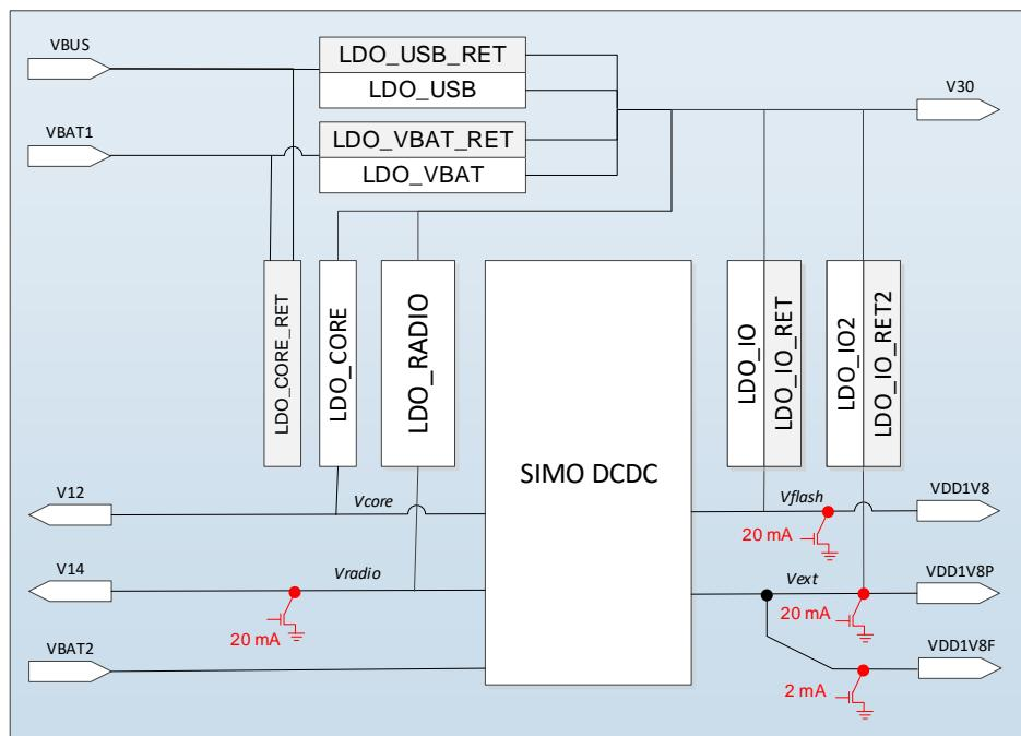
Figure 22. Power rail discharging feature
