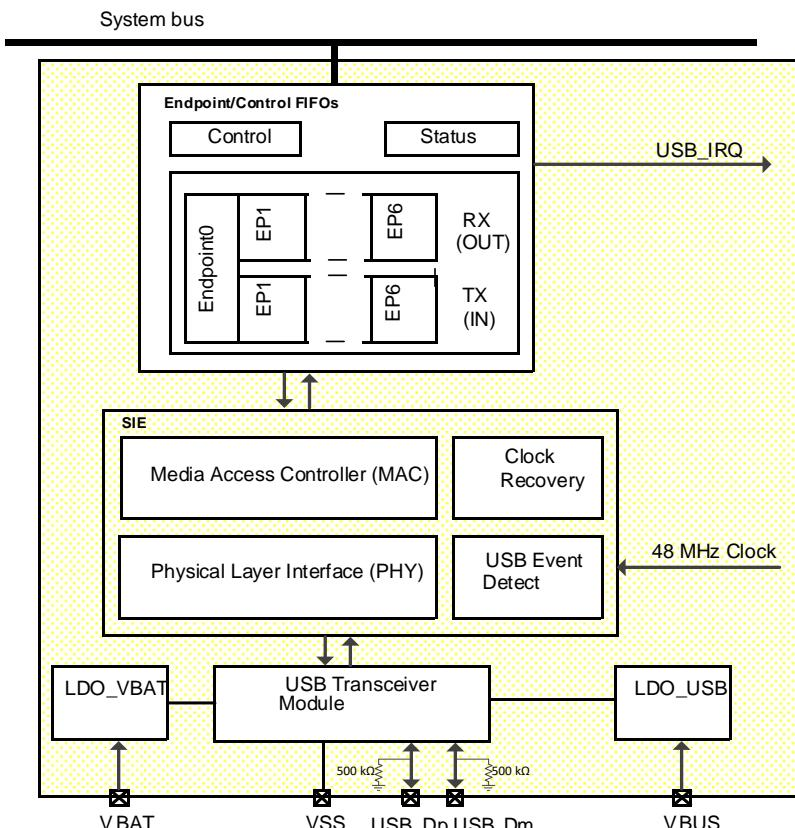
Figure 95. USB Node block diagram
