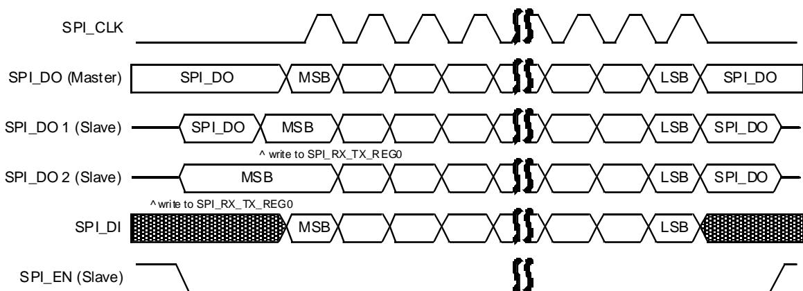
Figure 87. SPI Master/Slave mode 0: SPI\_POL=0 and SPI\_PHA=0
