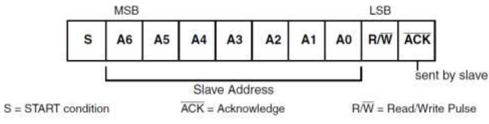
Figure 73. 7-bit address format
