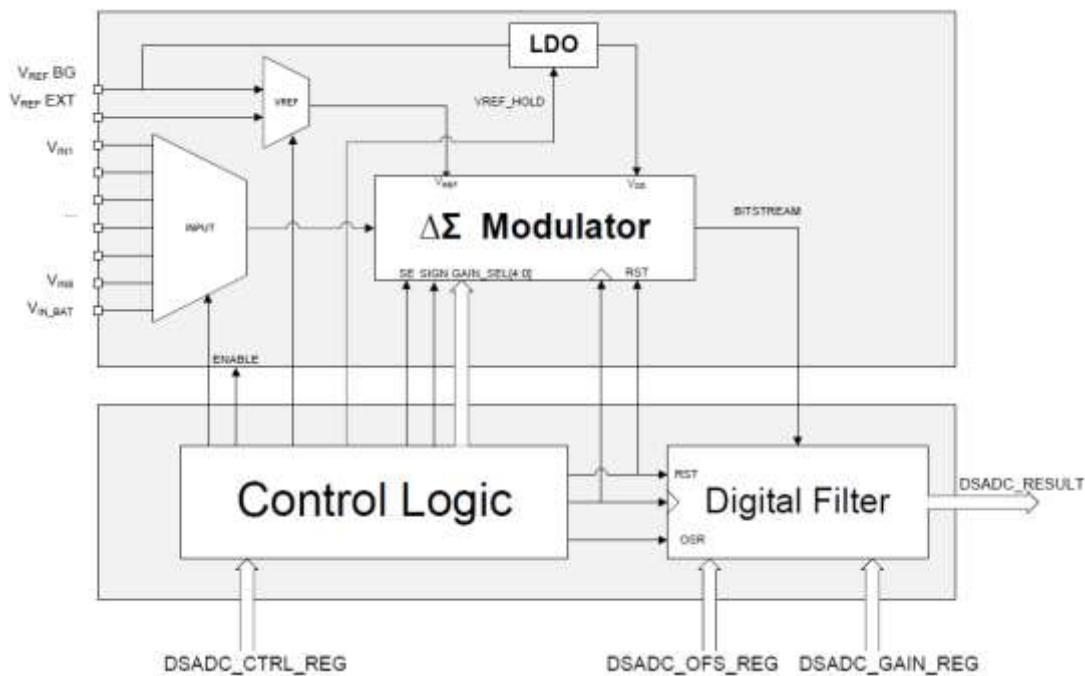
Figure 62. Block diagram of the  $\Delta\Sigma$  ADC
