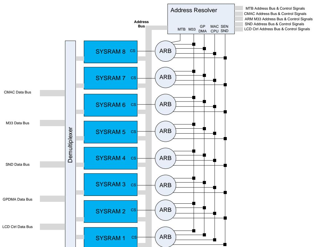
Figure 34. Internal architecture of the memory controller
