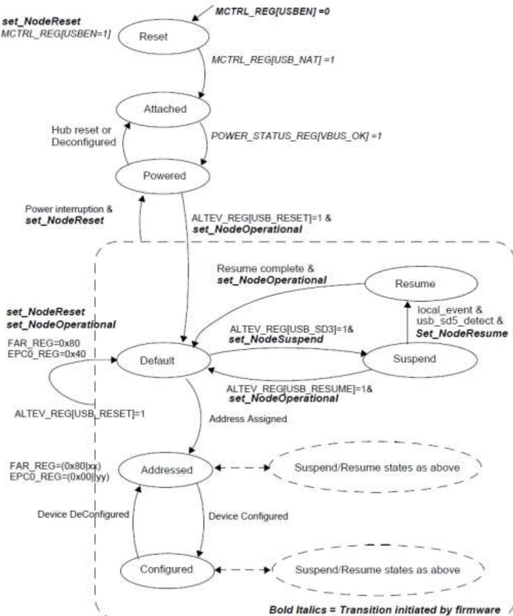
Figure 97. Node Functional State Diagram
