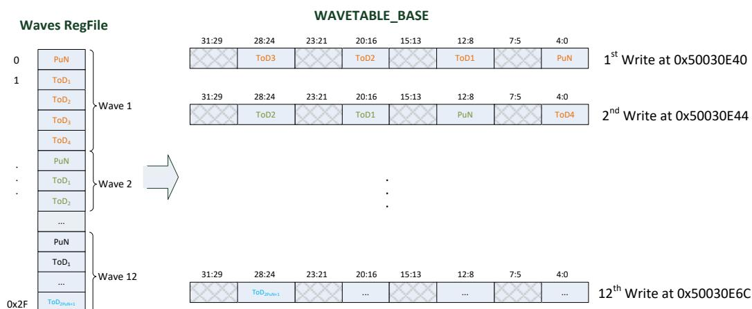
**Figure 50. Loading waves into waves memory space**
