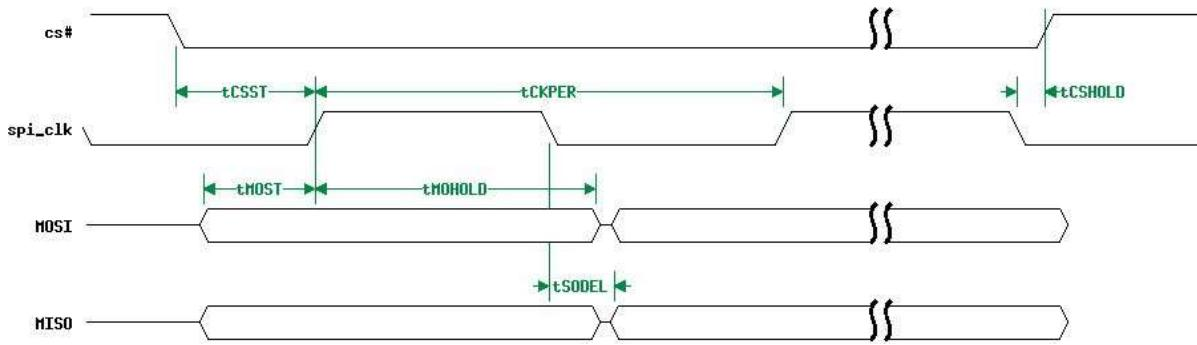
Figure 91. SPI Slave mode timing (CPOL = 0, CPHA = 0)
