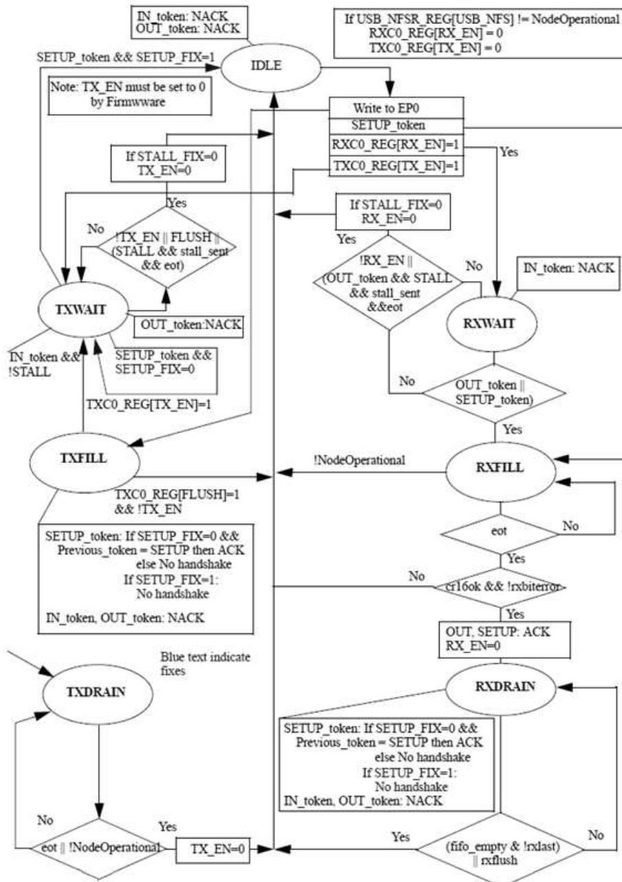
Figure 99. Endpoint 0 operation
