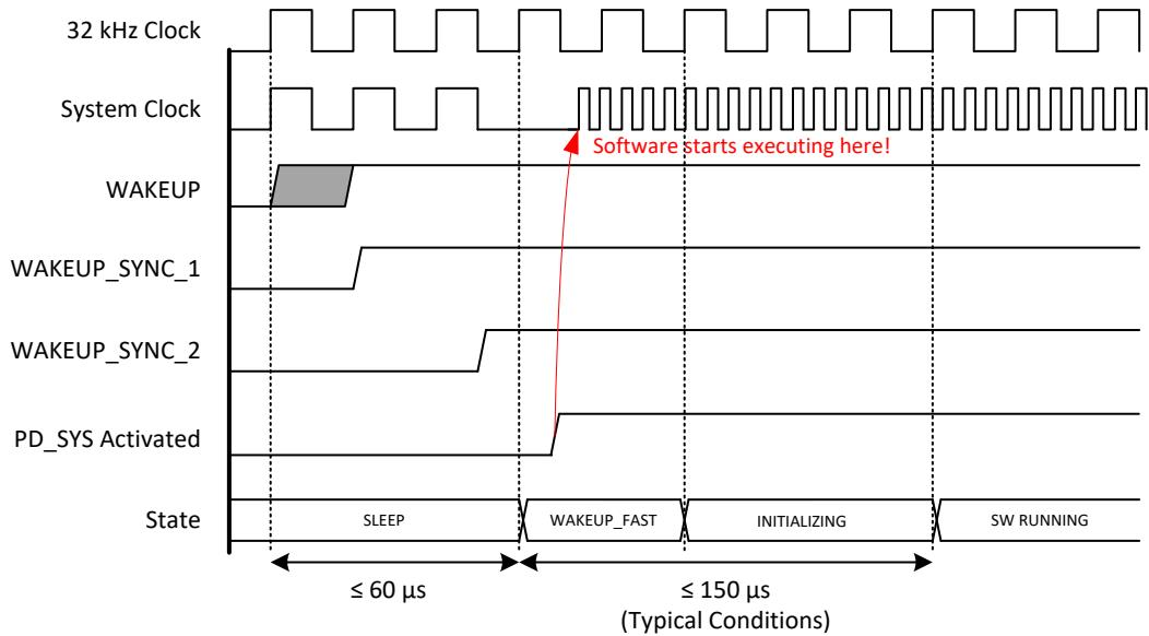
Figure 12. Ultra-fast wake-up timing
