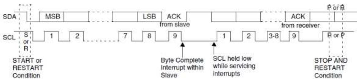
**Figure 71. Data transfer on the I2C bus**
