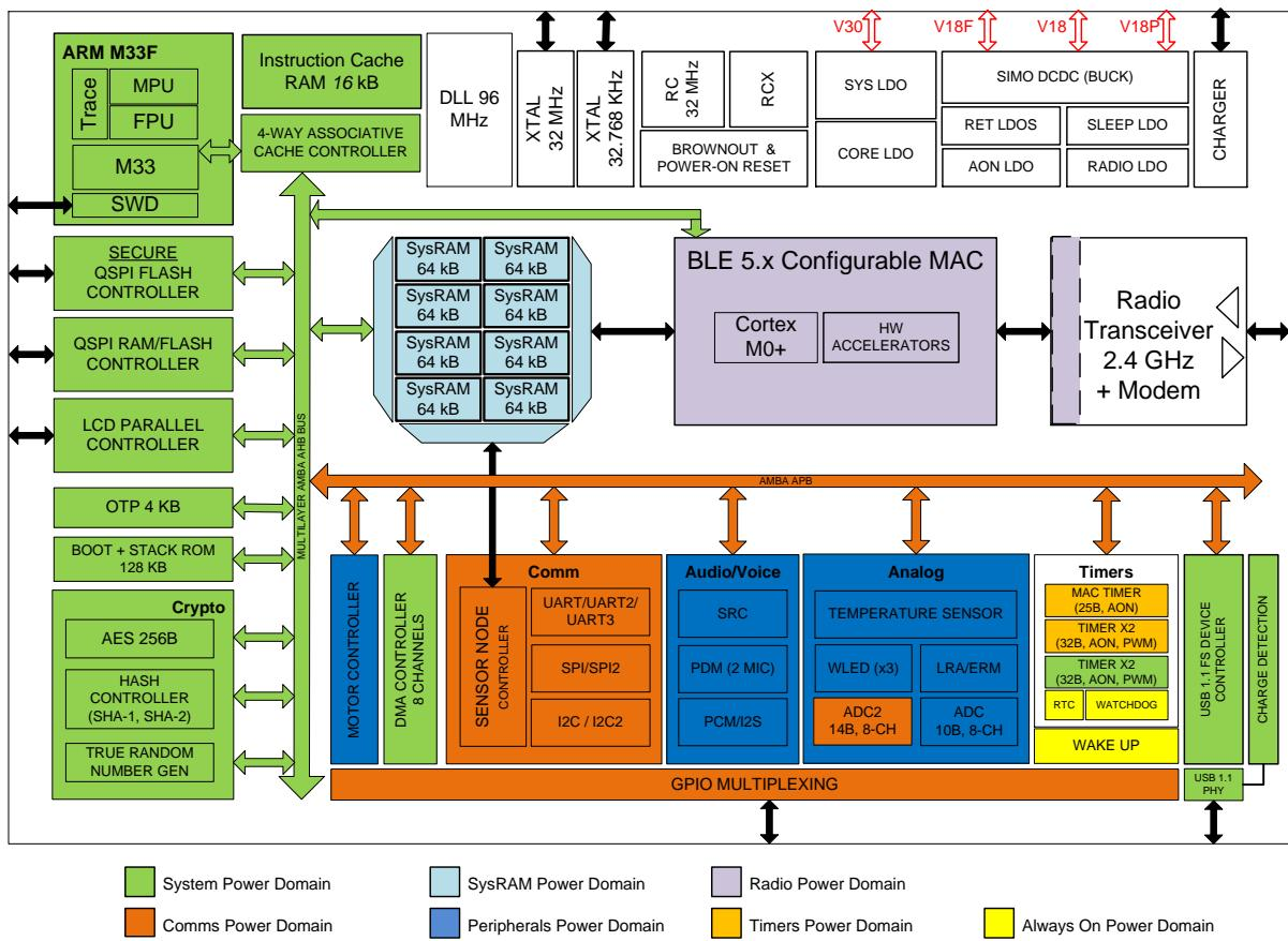
Figure 7. Digital power domains and blocks mapping
