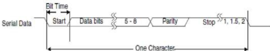
**Figure 81.** Serial data format
