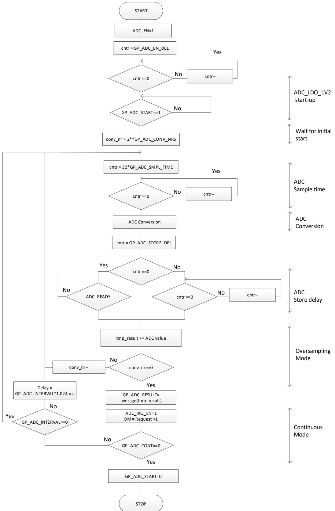
Figure 61. GPADC operation flow diagram
