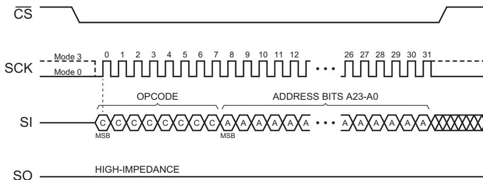
Figure 20. Block Erase Timing
