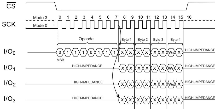
Figure 13. Set Burst with Wrap Timing (SPI Mode)
