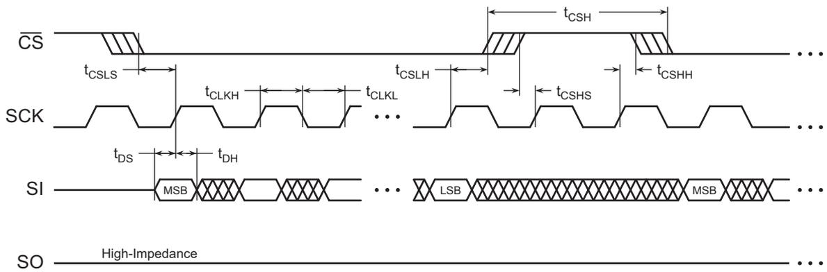
Figure 43. Serial Input Timing
