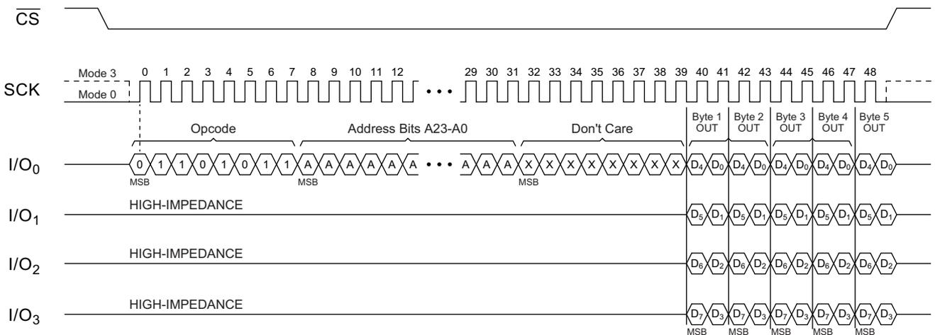
Figure 10. Quad-Output Fast Read Array
