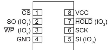
Figure 2. 8-DFN (5 x 6 and 2 x 3) — Top View
