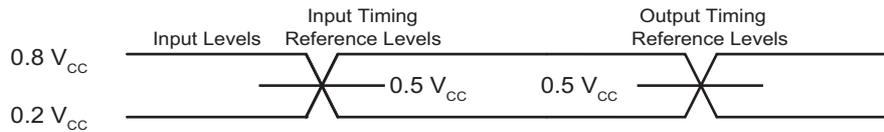
Figure 31. AC Measurement I/O Waveform
