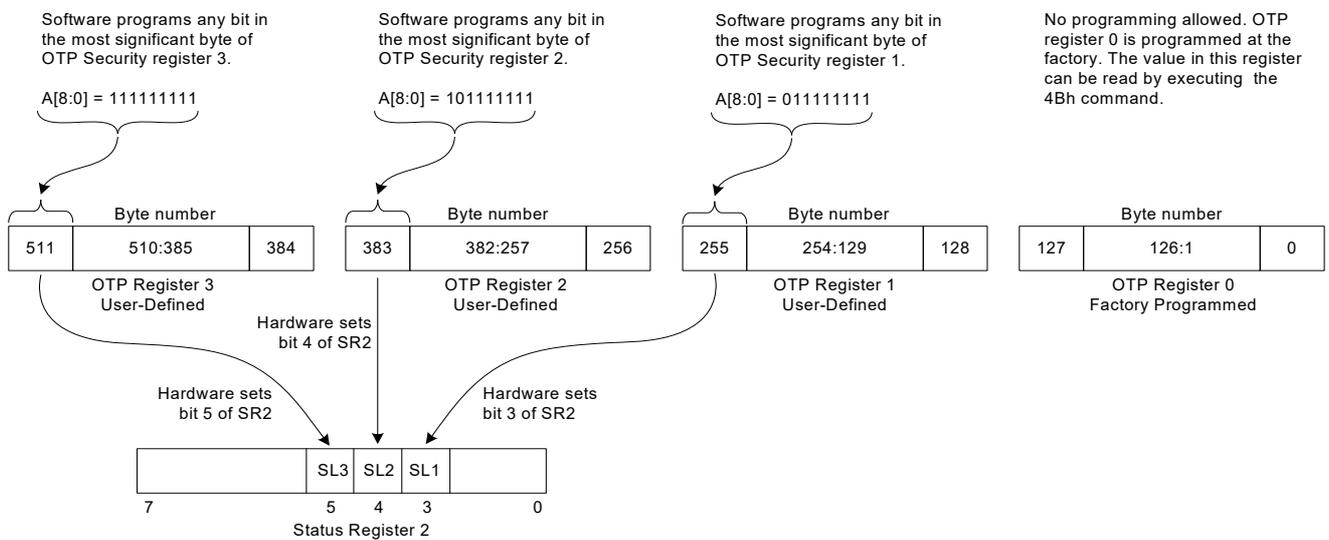
Figure 21. OTP Security Register Program and Lock
