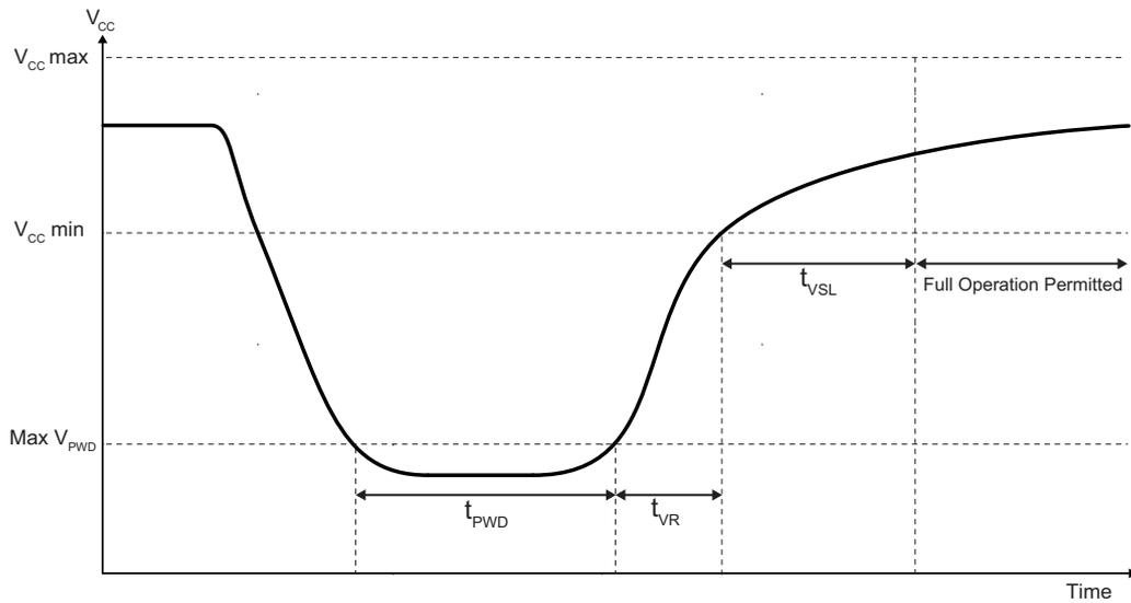
Figure 34. AC Power-up Timing After a Brown-Out
