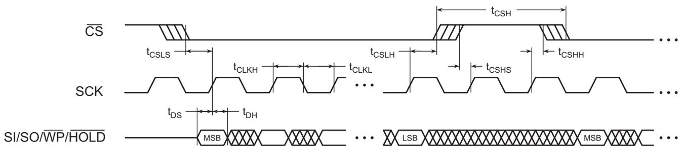
Figure 35. Serial Input Timing
