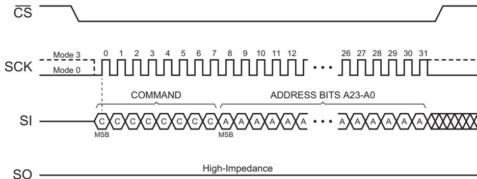
Figure 4. SPI Transfer — Command and Address Only
