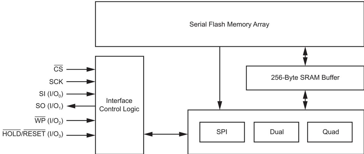
Figure 2. Block Diagram
