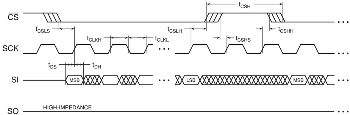
Figure 14-2. Serial Output Timing
