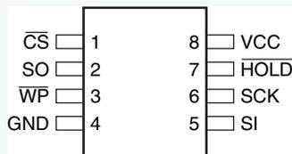
Figure 2-3. 8-UDFN (Top View)
