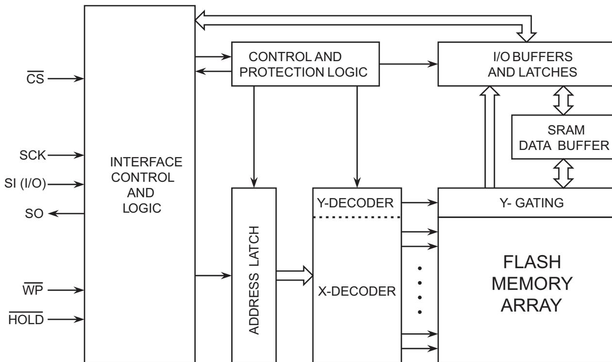
Figure 5. Block Diagram
