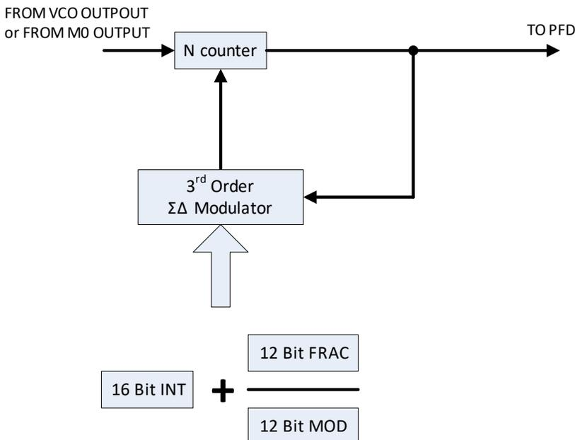
The 16 INT bits (Bit[D30:D15] in Register 0) set the integer part of the feedback division ratio.
