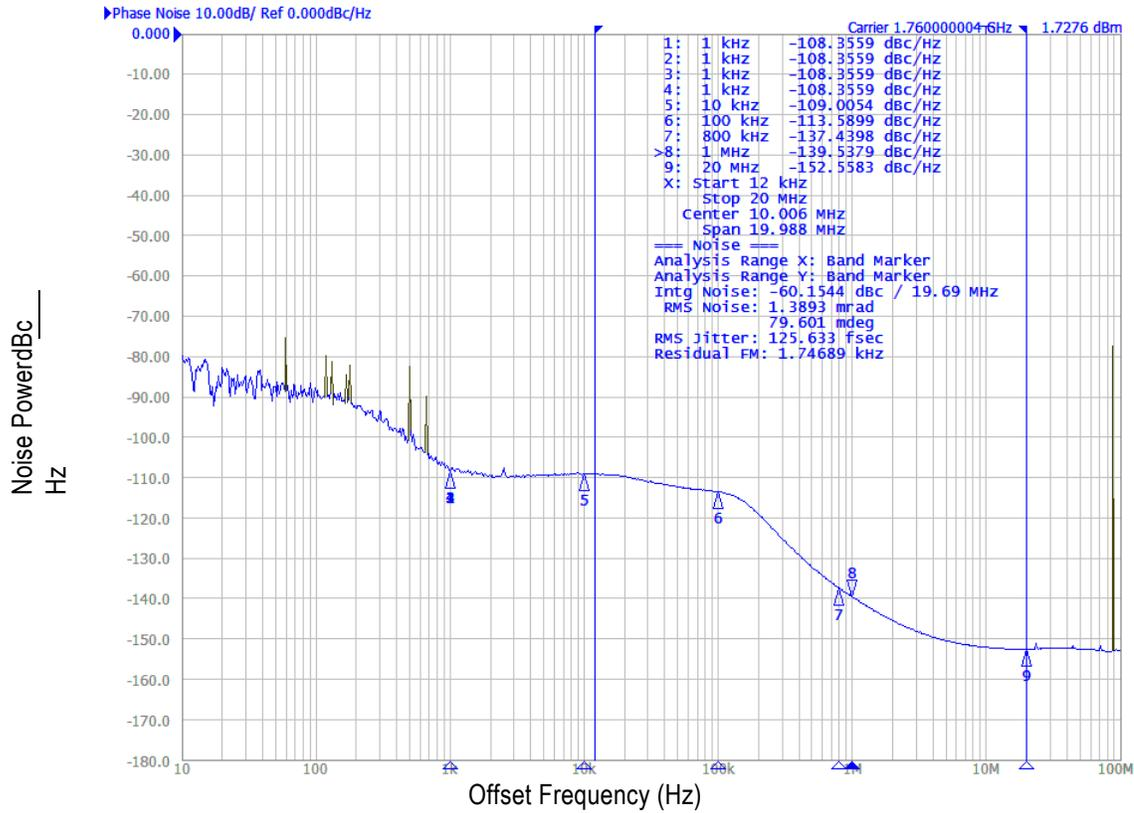
Phase Noise Performance (Open Loop) at 1.1GHz (3.3V)
