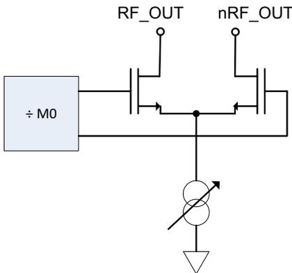
Eight programmable output power levels can be programmed from -4dBm to +7dBm (see [RF Output Power](#)).
