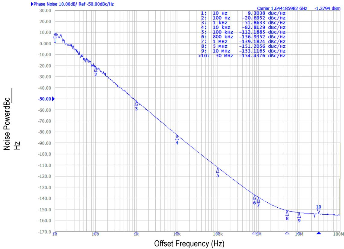
Phase Noise Performance (Open Loop) at 2.3GHz (3.3V)
