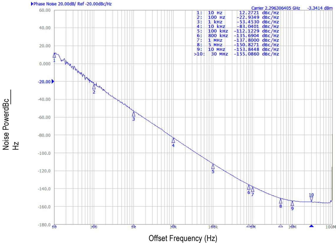
Phase Noise Performance (Open Loop) at 3.8GHz (3.3V)
