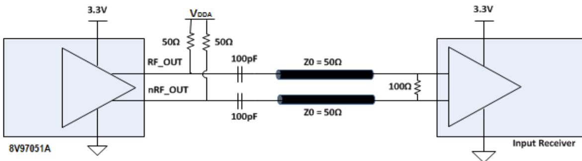
This termination scheme allows to provide one of the selected output power on the differential pair when connected to a 50Ω load. (See the [RF Output Power](#) for more information about the output power selection).
