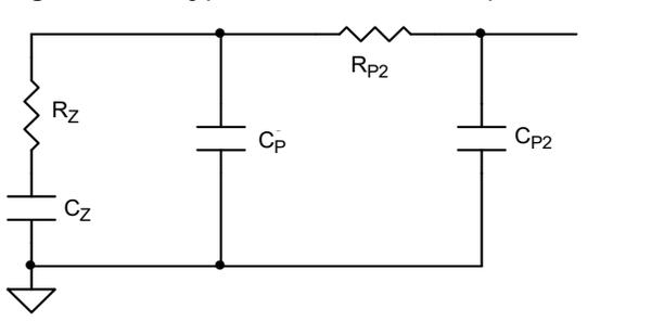
The  $R_z$ ,  $C_z$  and  $C_p$  can be calculated as 2<sup>nd</sup> order loop filter.
