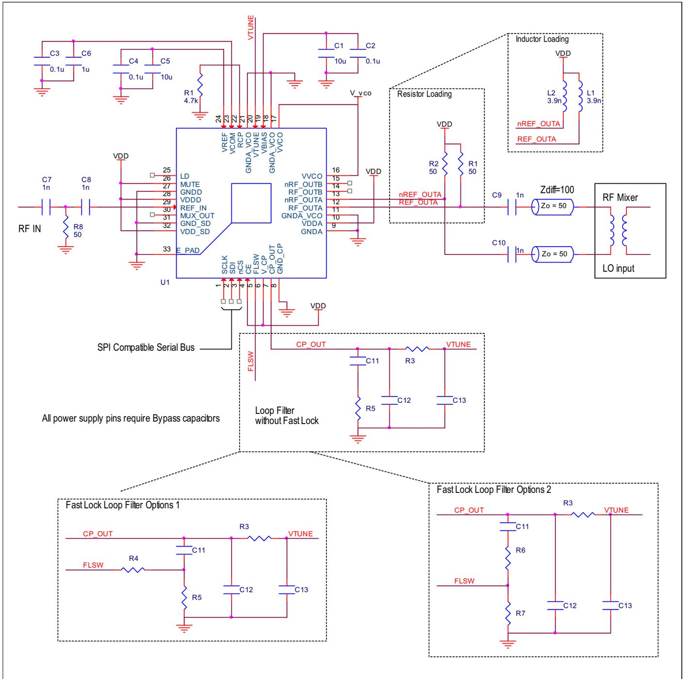
The 8V97051A output pull-up loading can be resistors or inductors. The pull up resistor value is typically 50Ω. Resistor pull up loading covers wide range of output frequencies. For inductor pull up loading, the inductor value is frequency dependent. One inductor value cannot cover all the output frequency range. This example shows the  $L = 3.9\text{nH}$  that is suitable for approximately 2GHz operating frequency. The output can also drive single ended LO input.
