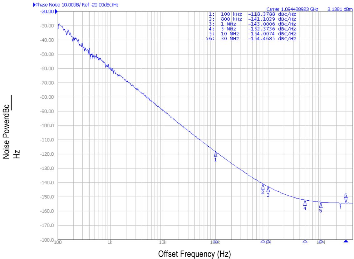
Phase Noise Performance (Open Loop) at 1.65GHz (3.3V)
