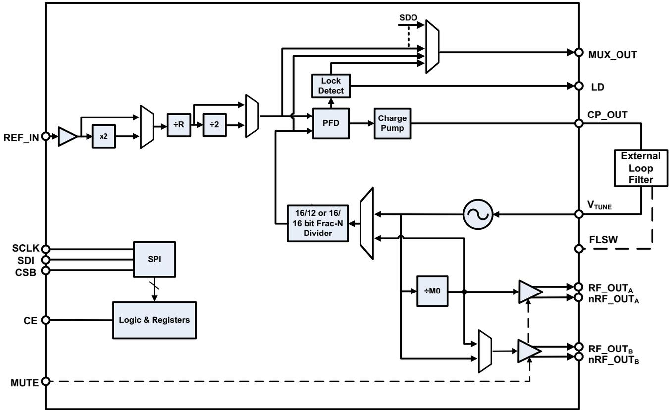
Note: 16-Bit Integer / 16-Bit Fractional feedback divider is available when using [Register 6](#).
