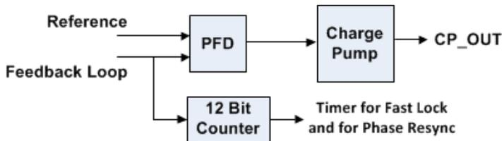
After the user program a frequency, the second sync pulse coming from the 12-bit counter, after the nCS is asserted high, is used to resynchronize the output phase to the input phase. To ensure that the PLL is locked before to resynchronize the output phase,  $T_{\text{SYNC}}$  must be larger than the worst case lock time.
