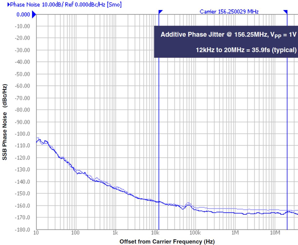
As with most timing specifications, phase noise measurements have issues relating to the limitations of the equipment. Often the noise floor of the equipment is higher than the noise floor of the device. This is illustrated above. The device meets the noise floor of what is shown, but can actually be lower. The phase noise is dependent on the input source and measurement equipment.
