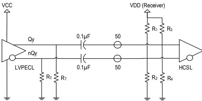
Figure 7. LVPECL Output AC-Coupled into HCSL Receiver
