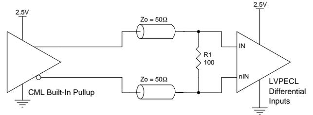
Figure 9. IN/nIN Input Driven by a 2.5V LVPECL Driver with AC Couple
