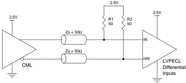
Figure 6. ON/nIN Input Driven by a 2.5V LVPECL Driver
