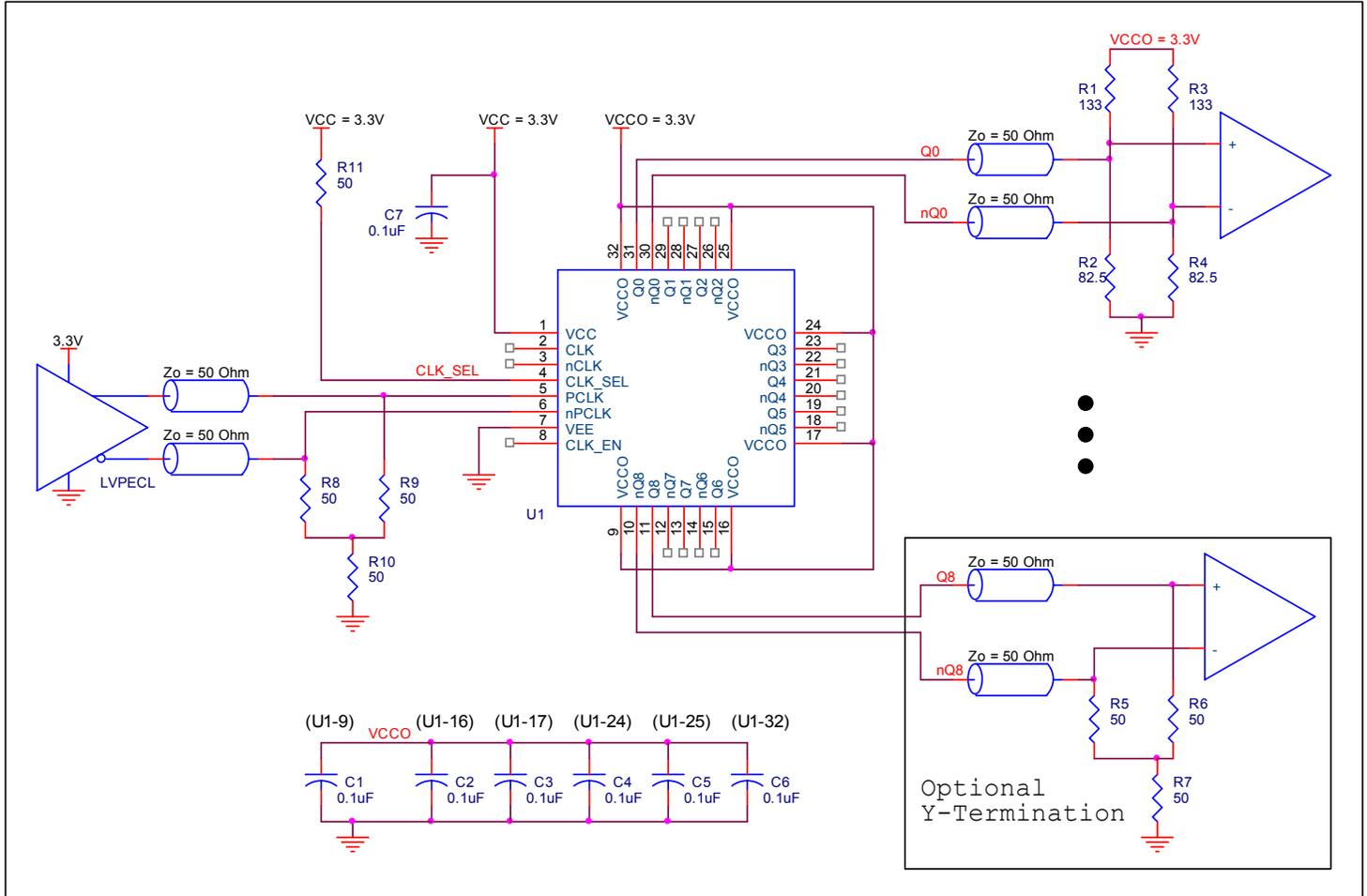
Figure 7. ICS853S0311 Example LVPECL Clock Output Buffer Schematic
