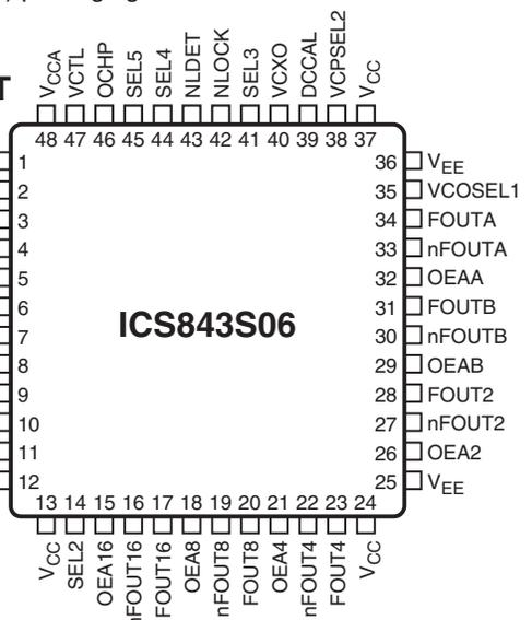
**48-Lead TQFP, E-Pad**
