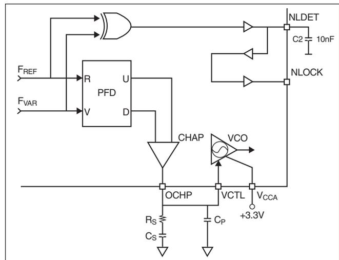
FIGURE 1. APPLICATION DIAGRAM
