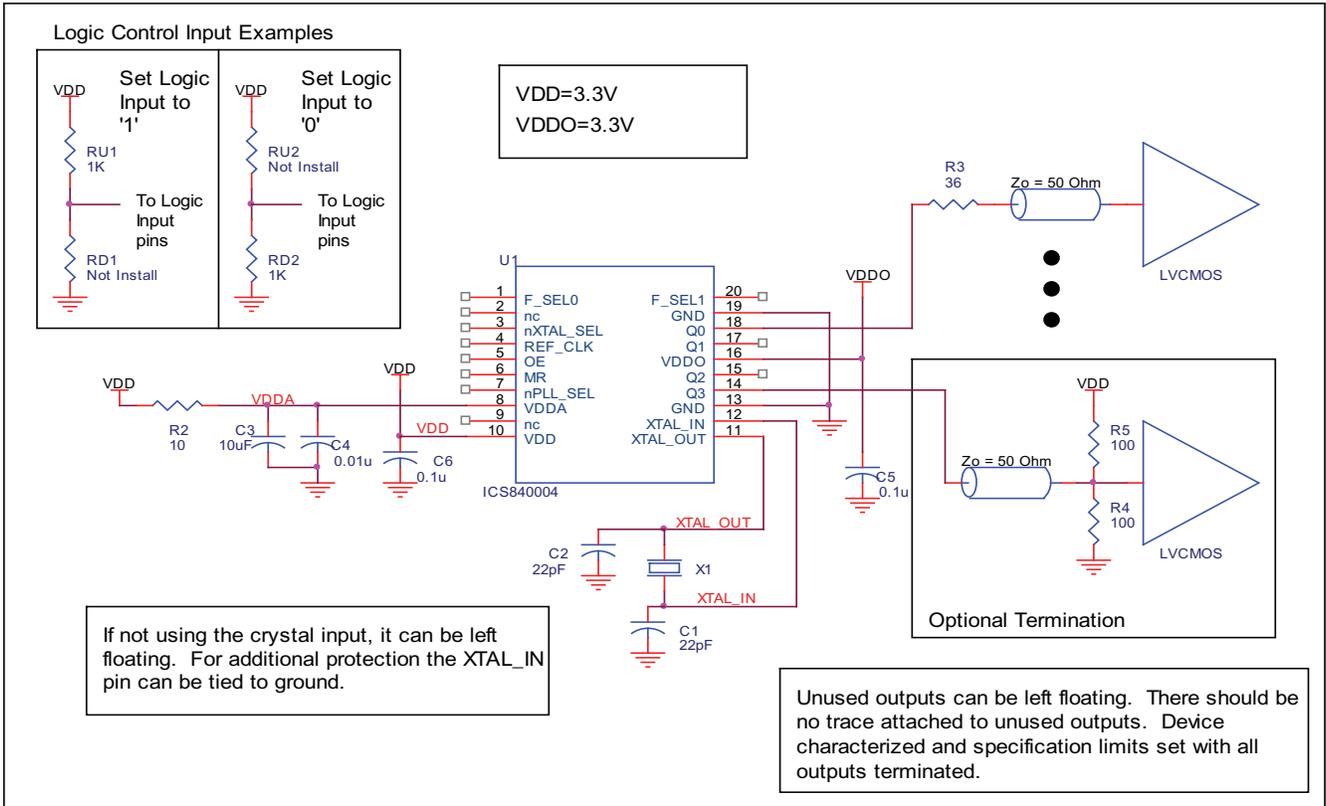
**FIGURE 4. 840004 SCHEMATIC EXAMPLE**
