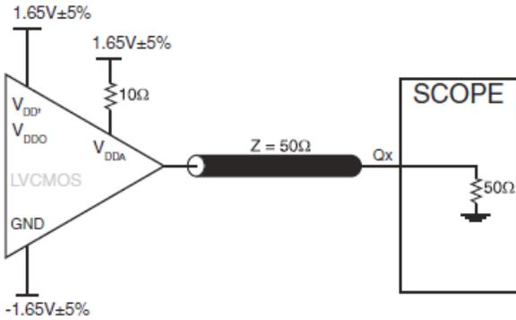
3.3V CORE/3.3V OUTPUT LOAD AC TEST CIRCUIT
