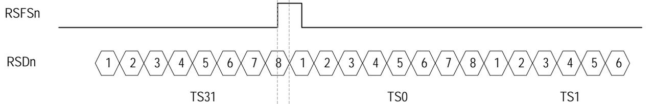
When the DE (b4, E1-010H) is logic 1 and the FE (b3, E1-010H) is logic 1:
