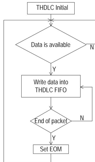
**Figure 80. Writing Data to T1/J1 Mode THDLC FIFO**
