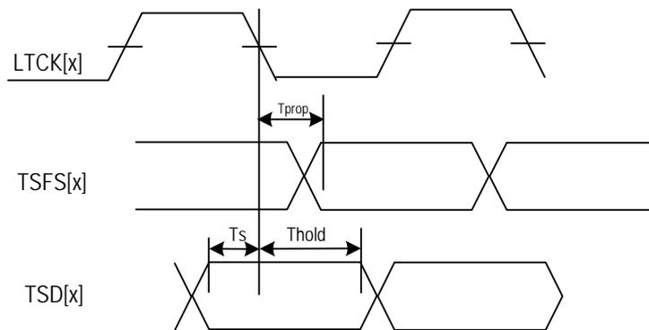
**Figure 90. Transmit Interface Timing (Line Transmit Clock)**
