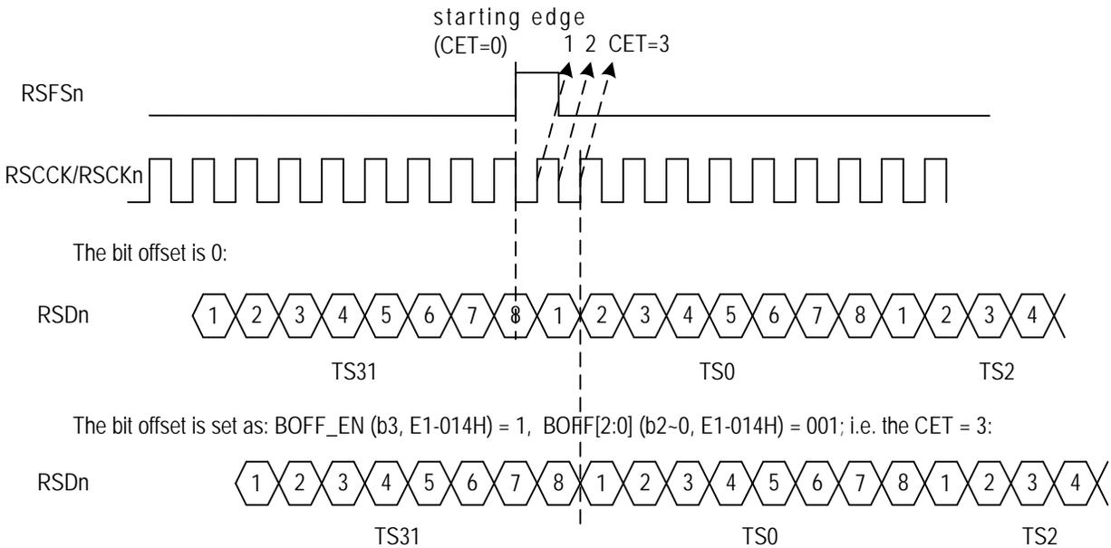
**Figure 23. Receive Bit Offset - Between RSFSn & RSDn**
