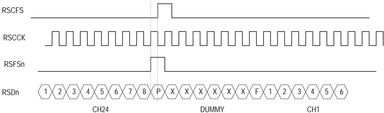
(The 'X' represent the filled bits and has no meaning.)
