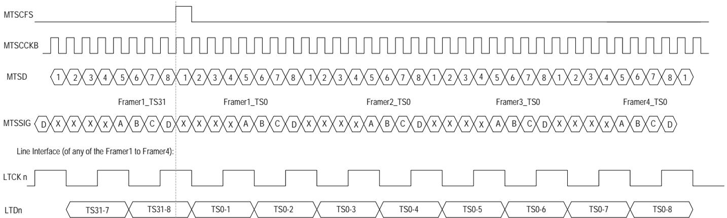
**Figure 46. E1 Transmit Multiplexed Mode - Functional Timing Example 1**
