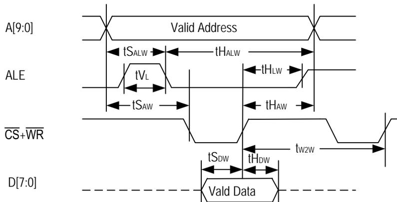
**Figure 88. Write Access Timing**
