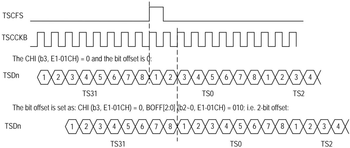
Figure 48. Transmit Bit Offset in E1 Mode - 1
