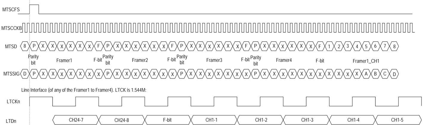
**Figure 62. T1/J1 Transmit Multiplexed Mode - Functional Timing Example 2**
