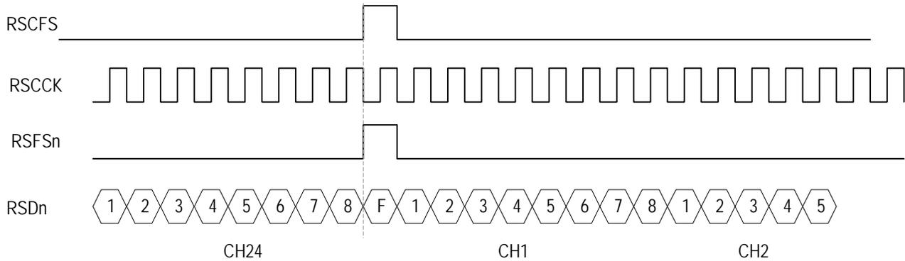
(The RSCKn is selected by the RSCKSEL (b5, T1/J1-001H) to output a jitter attenuated 1.544MHz (i.e., smoothed LRCKn) or 8KHz clock (smoothed LRCKn divided by 193).)
