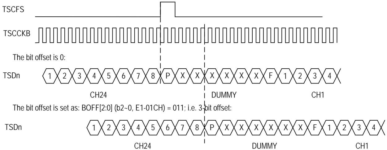
**Figure 64. Transmit Bit Offset in T1/J1 Mode - 2**
