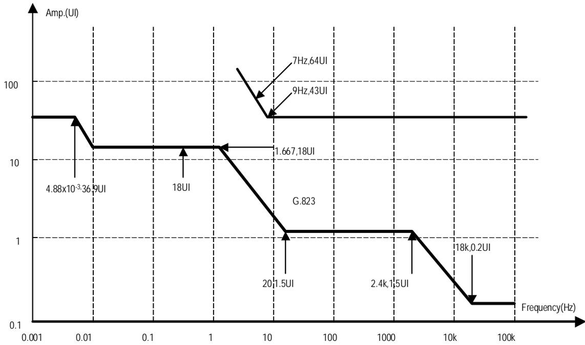
Figure 65. E1 Mode Jitter Tolerance ( $N1 = N2 = 2fH$ )
