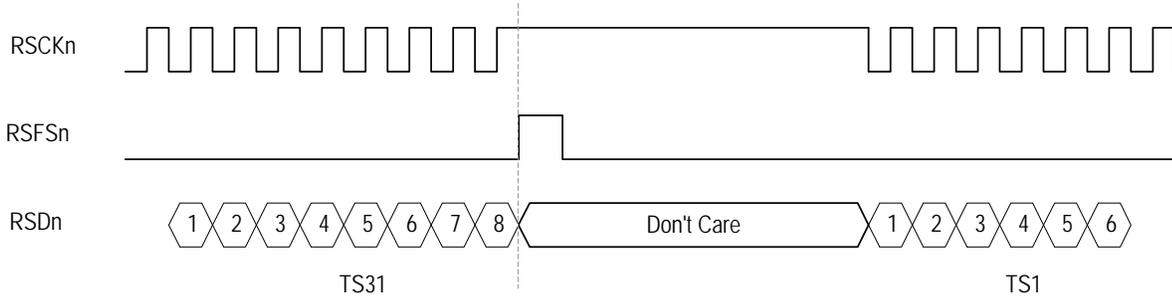
When the DE (b4, E1-010H) is logic 1 and the FE (b3, E1-010H) is logic 0:
