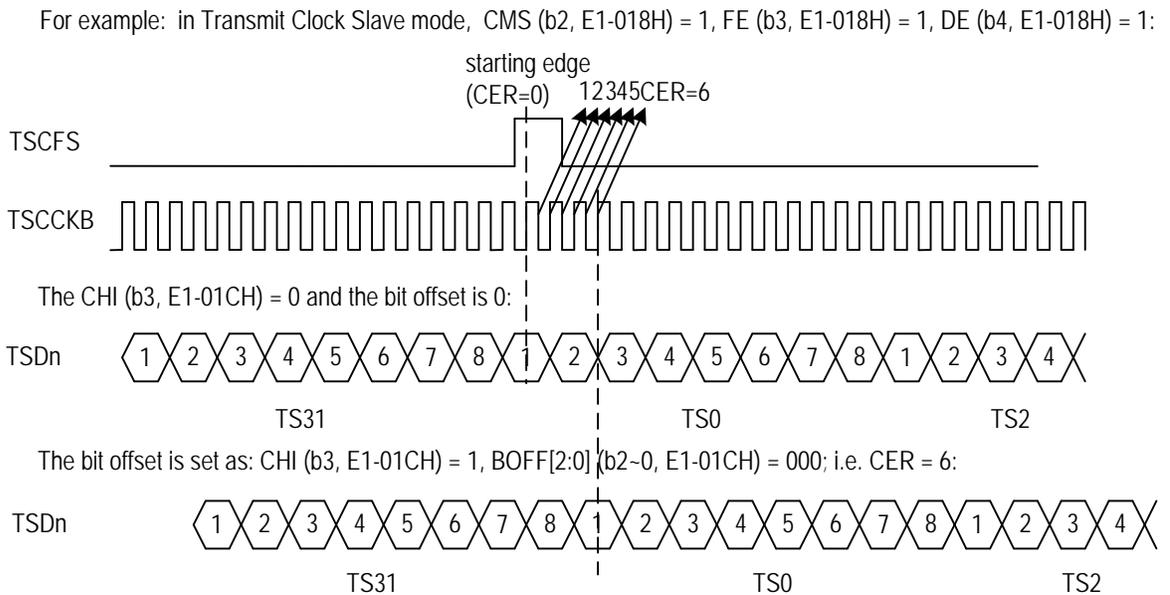
**Figure 51. Transmit Bit Offset in E1 Mode - 4**
