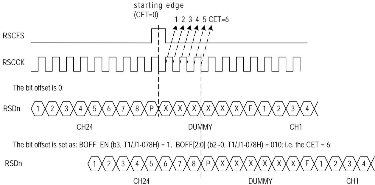
**Figure 35. Receive Bit Offset in T1/J1 Mode**
