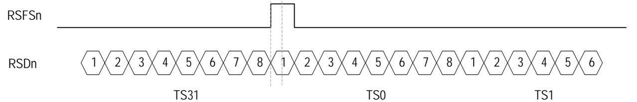
**Figure 16. E1 Receive Clock Master Full E1 Mode - Functional Timing Example**
