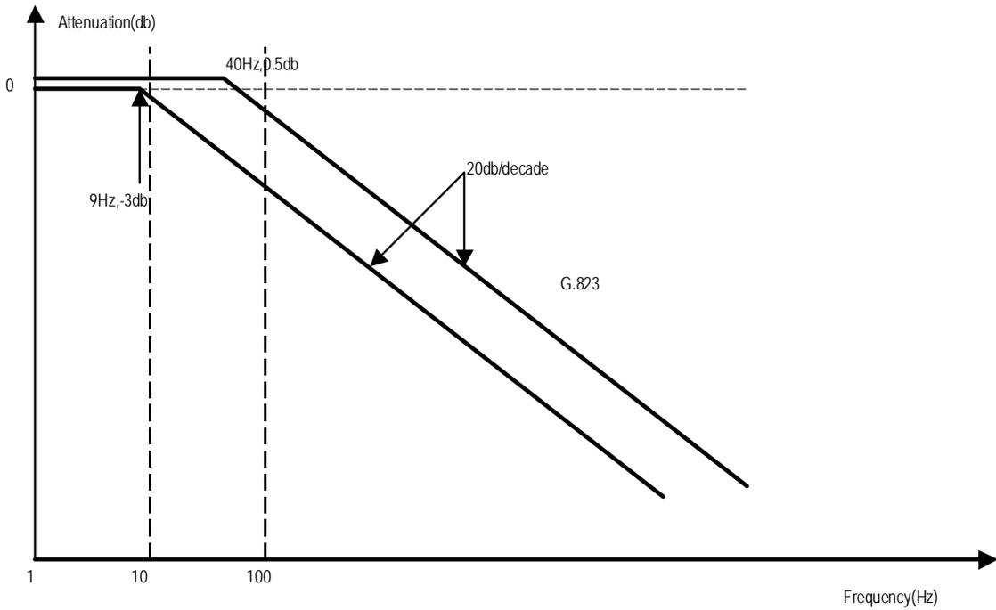
Figure 66. E1 Mode Jitter Transfer ( $N1 = N2 = 2fH$ )
