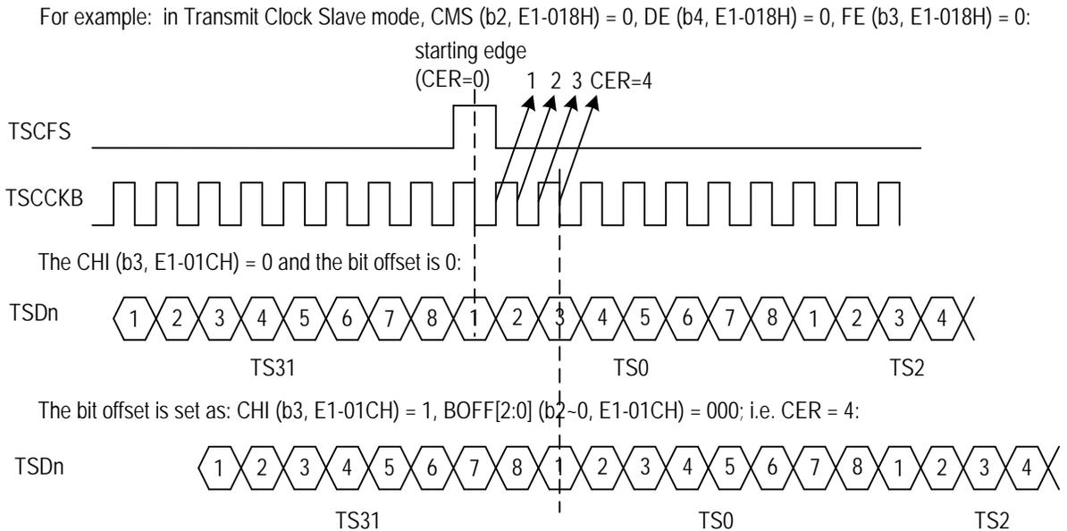
**Figure 50. Transmit Bit Offset in E1 Mode - 3**
