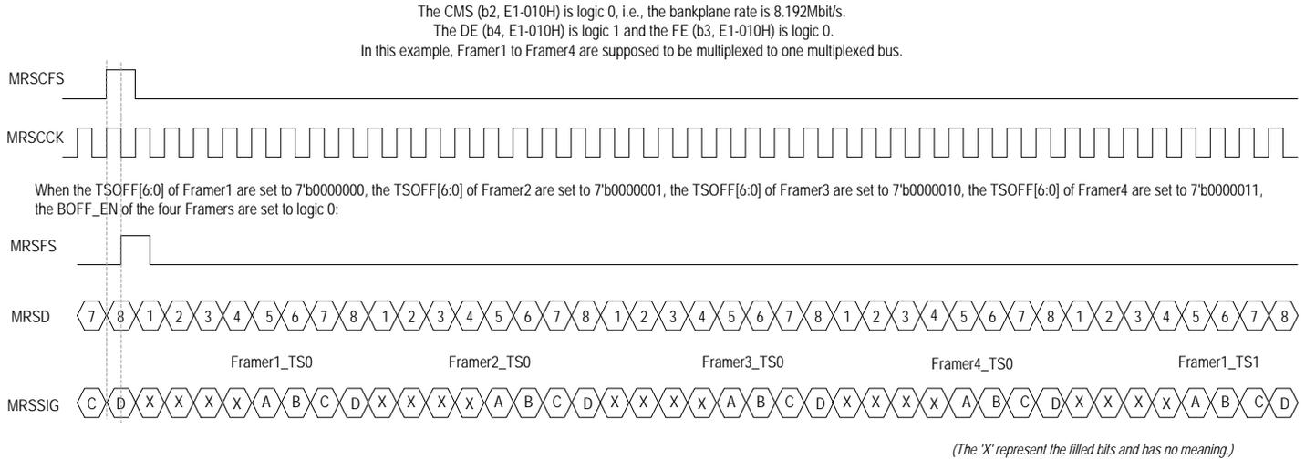
**Figure 20. E1 Receive Multiplexed Mode - Functional Timing Example 1**
