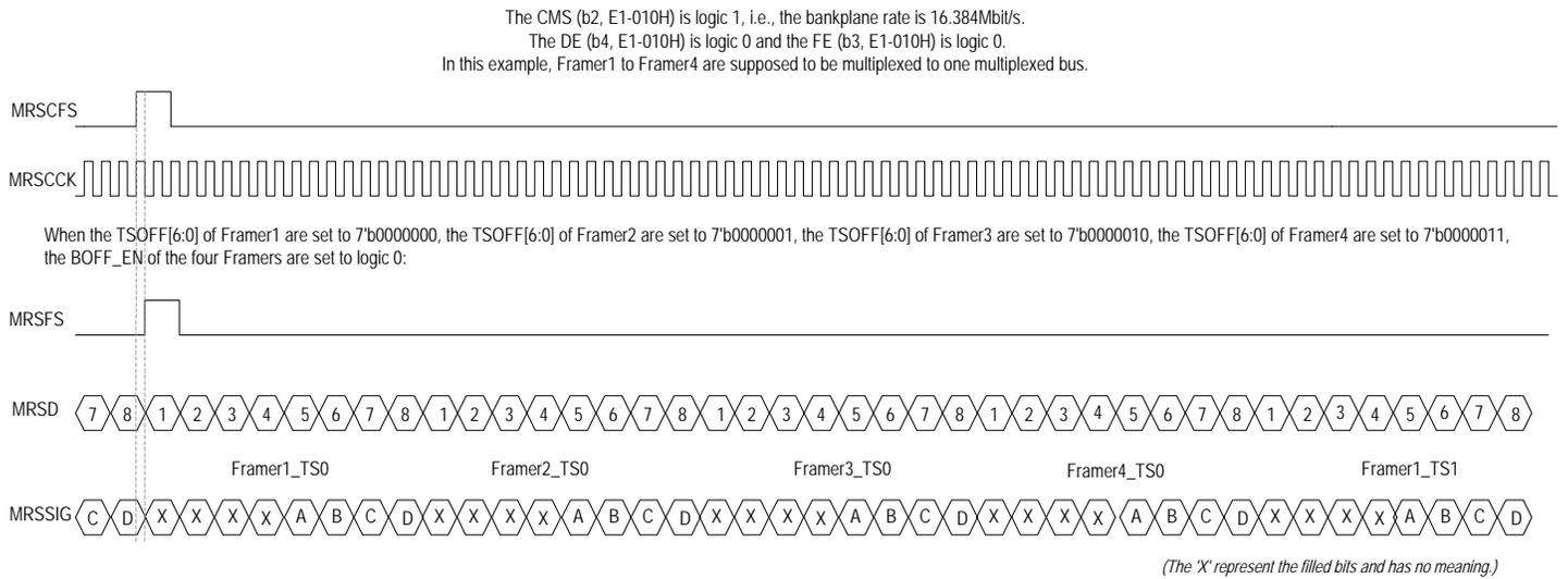
**Figure 21. E1 Receive Multiplexed Mode - Functional Timing Example 2**
