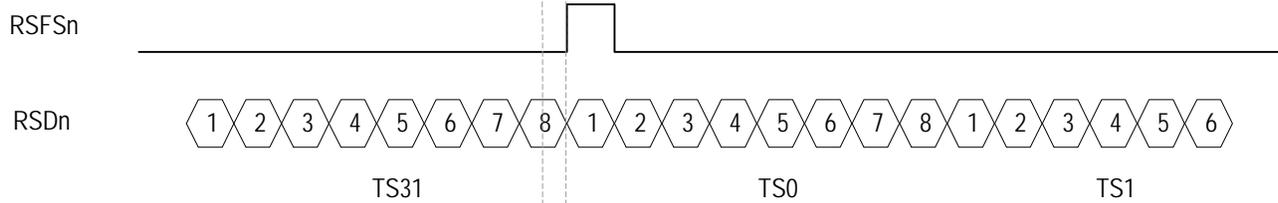
When the DE (b4, E1-010H) is logic 1 and the FE (b3, E1-010H) is logic 0:
