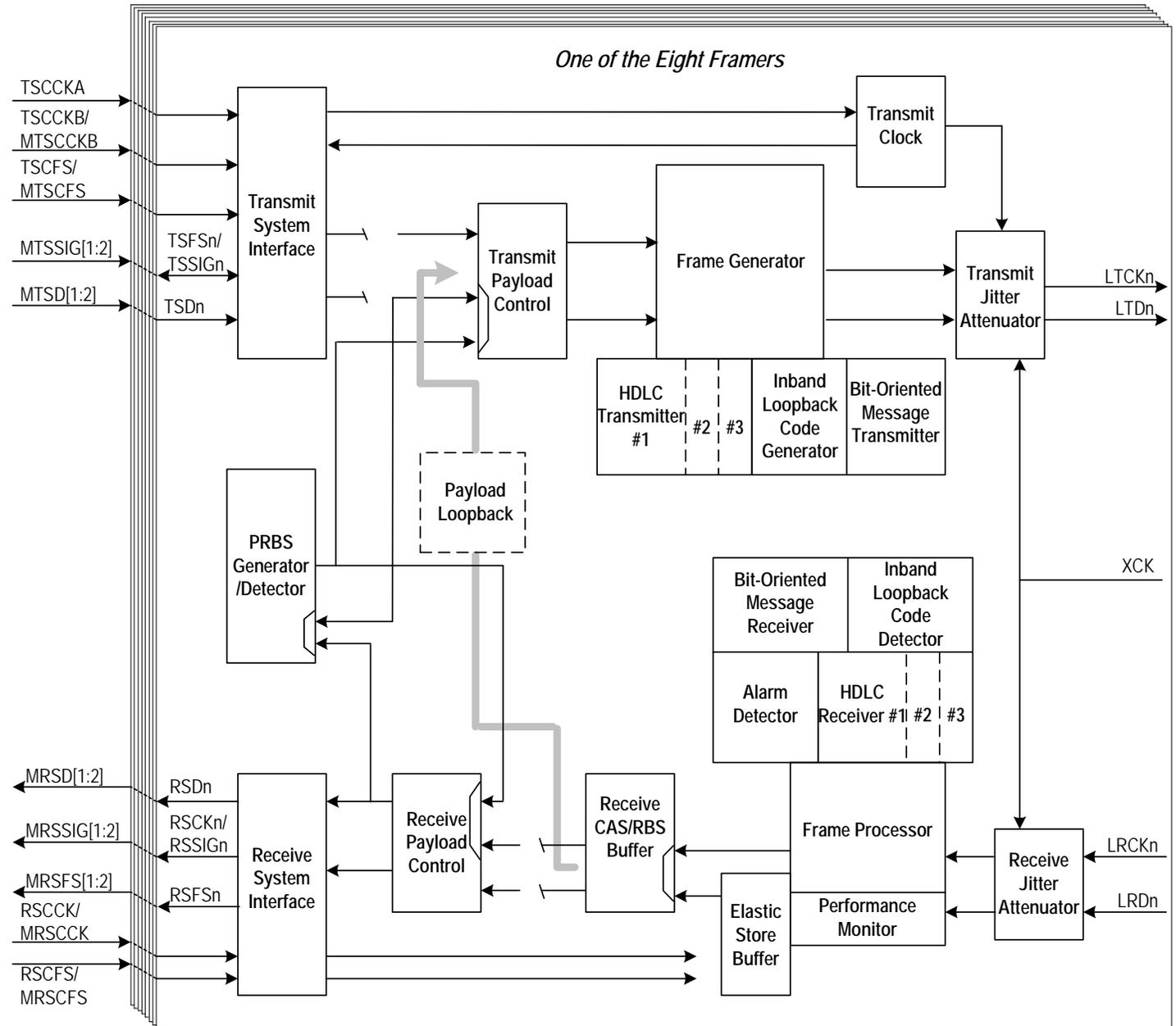
Figure 72. Payload Loopback
