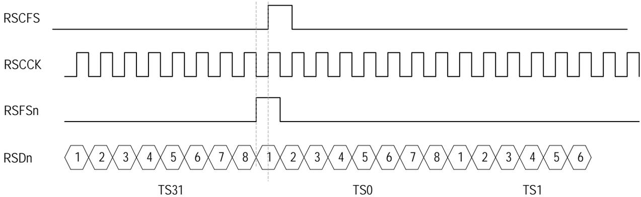
(The RSCCKn is selected by the RSCCKSEL (b5, E1-001H) to output a jitter attenuated 2.048MHz (i.e., smoothed LRCKn) or 8KHz clock (smoothed LRCKn divided by 256).)
