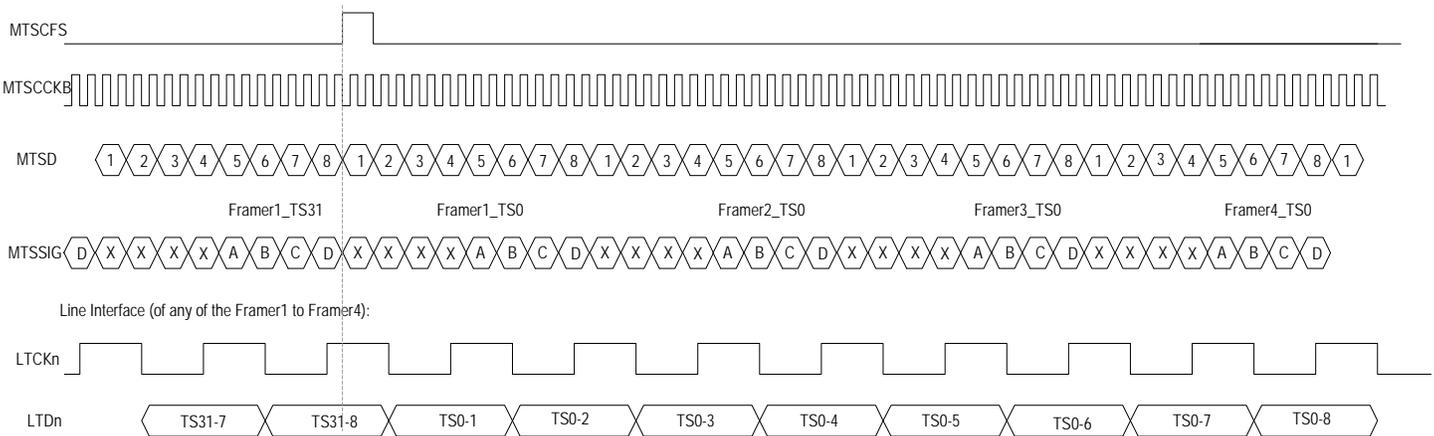
**Figure 47. E1 Transmit Multiplexed Mode - Functional Timing Example 2**
