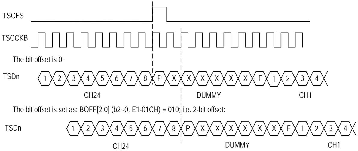
**Figure 63. Transmit Bit Offset in T1/J1 Mode - 1**
