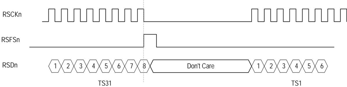
When the DE (b4, E1-010H) is logic 0 and the FE (b3, E1-010H) is logic 1:
