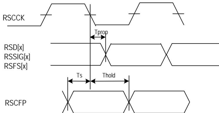
Figure 91. Receive Interface Timing (Receive System Common Clock)
