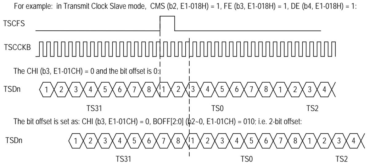
Figure 49. Transmit Bit Offset in E1 Mode - 2
