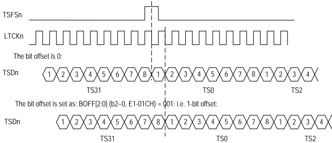
**Figure 52. Transmit Bit Offset in E1 Mode - 5**
