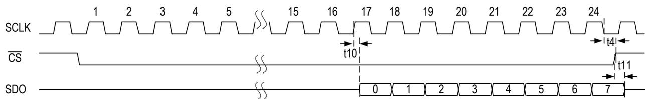
Figure-32 Serial Interface Read Timing with SCLKE=0
