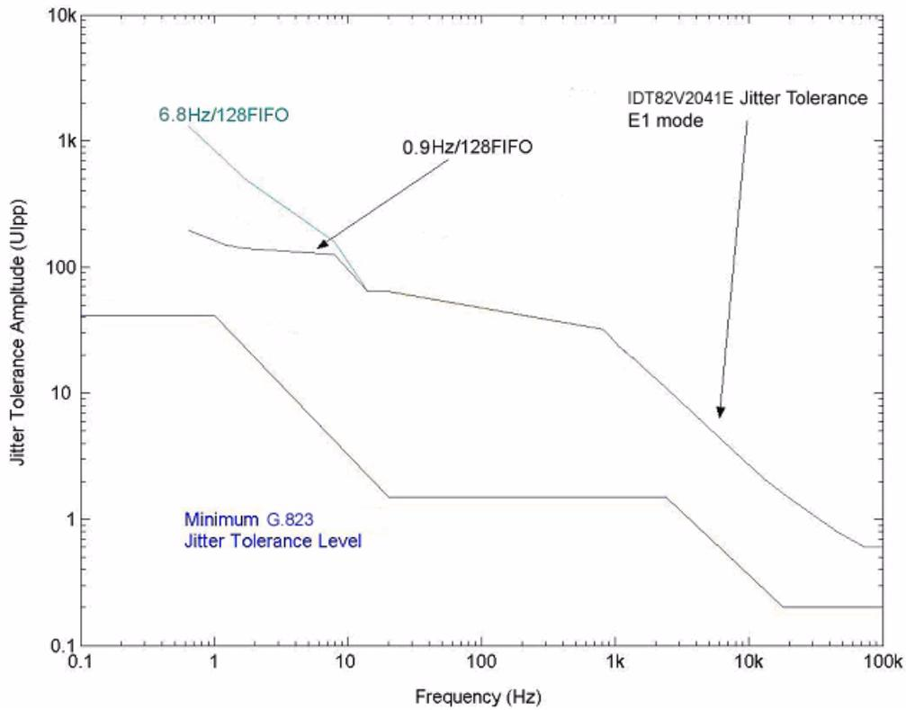
Figure-22 E1 Jitter Tolerance Performance
