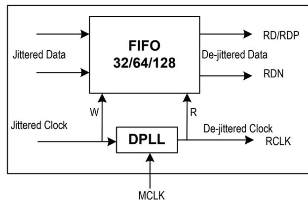
**Figure-11 Jitter Attenuator**
