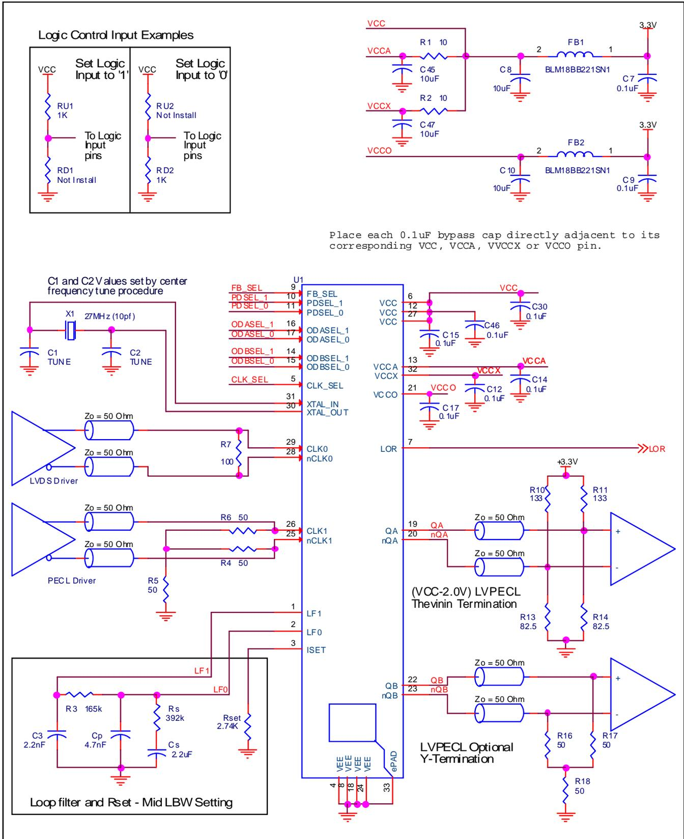
Place each 0.1uF bypass cap directly adjacent to its corresponding VCC, VCCA, VCCX or VCCO pin.
