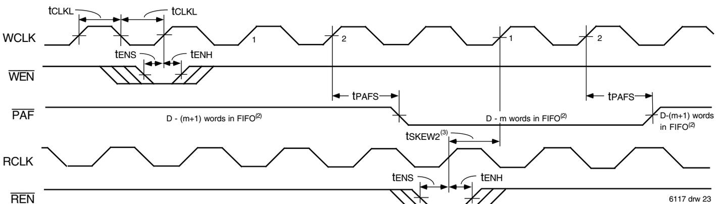
Figure 18. Synchronous Programmable Almost-Full Flag Timing (Standard and FWFT Modes)
