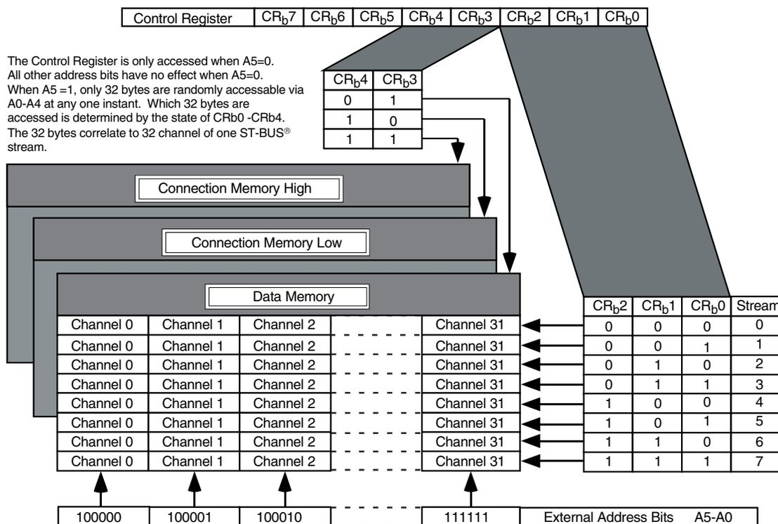
Figure 3. Address Mapping
