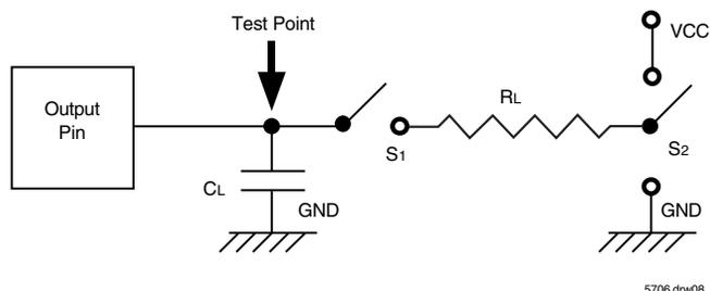
Figure 4. Output Load
