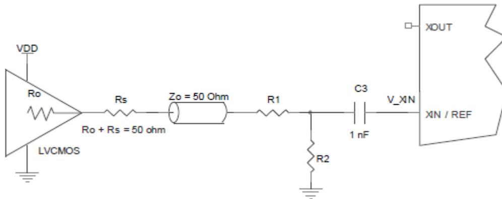
Figure 10. Overdriving XIN with a CMOS Driver
