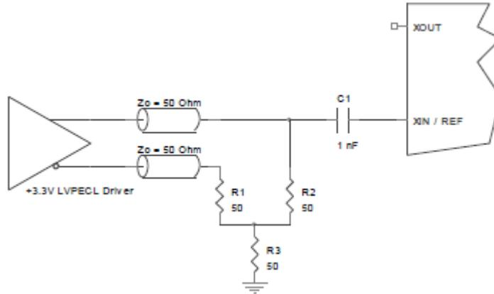
Figure 11. Overdriving XIN with an LVPECL Driver
