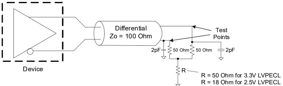
Figure 6. LVPECL Test Load
