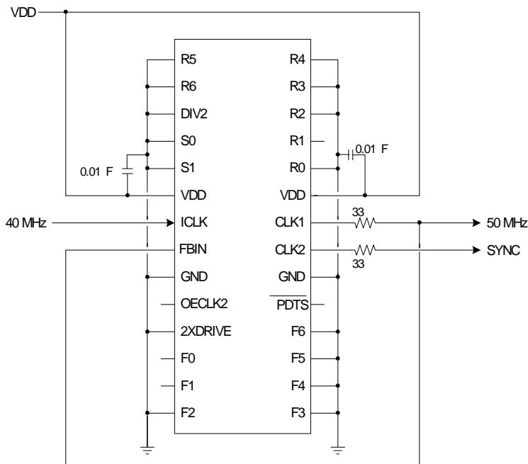
Note: The series termination resistor is located before the feedback trace.
