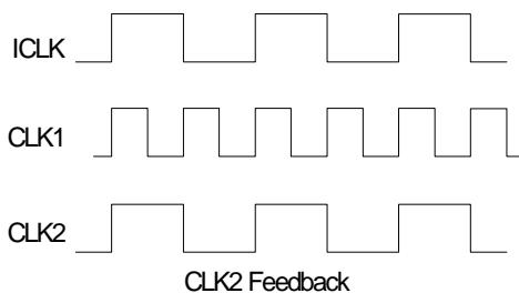
Using CLK1 as feedback will always result in synchronized rising edges between ICLK and CLK1 if CLK1 is used as feedback. CLK2 could be a falling edge compared to ICLK. Therefore, wherever possible, it is recommended to use CLK2 for feedback, which will synchronize the rising edges of all three clocks.
