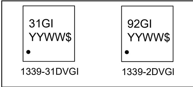
**Marking Diagram (16-SOIC)**
