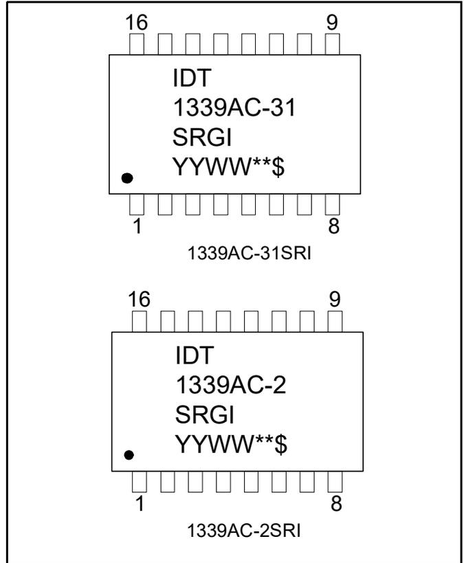
**Marking Diagram (8-SOIC)**
