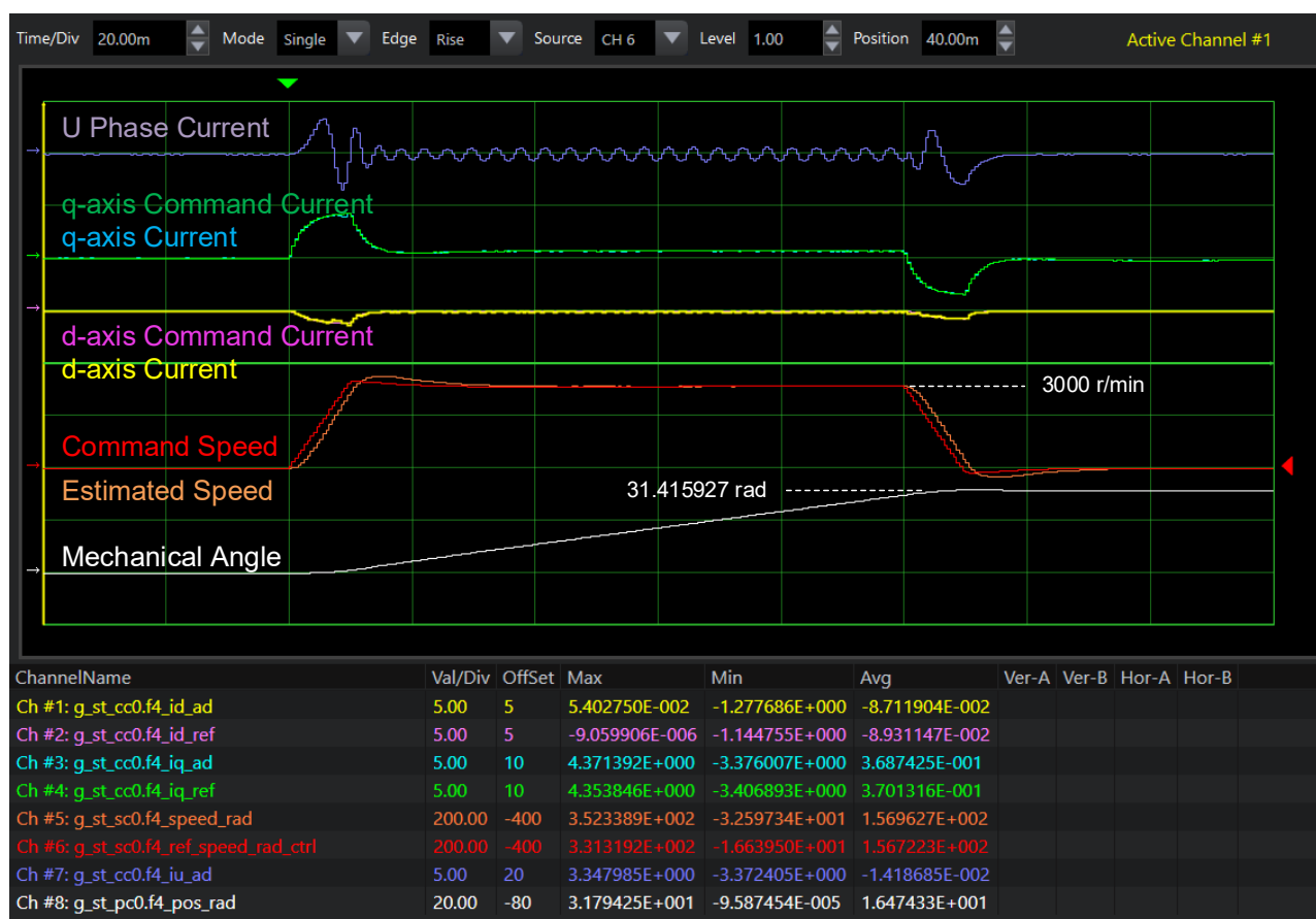
Figure 11-1 Acceleration and deceleration characteristics.
