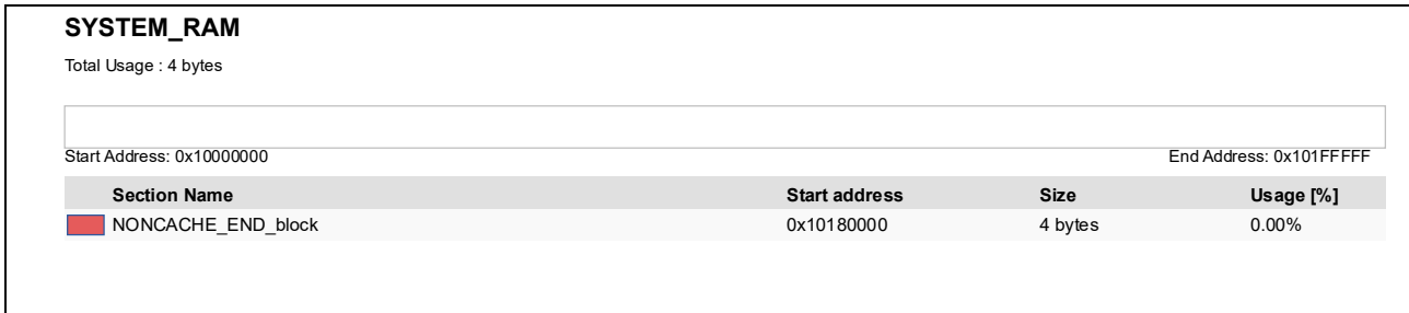
Figure 8.53. SYSTEM_RAM footprint of the RZ/T2H, N2H (CR52_dual) Primary project (EWARM)
