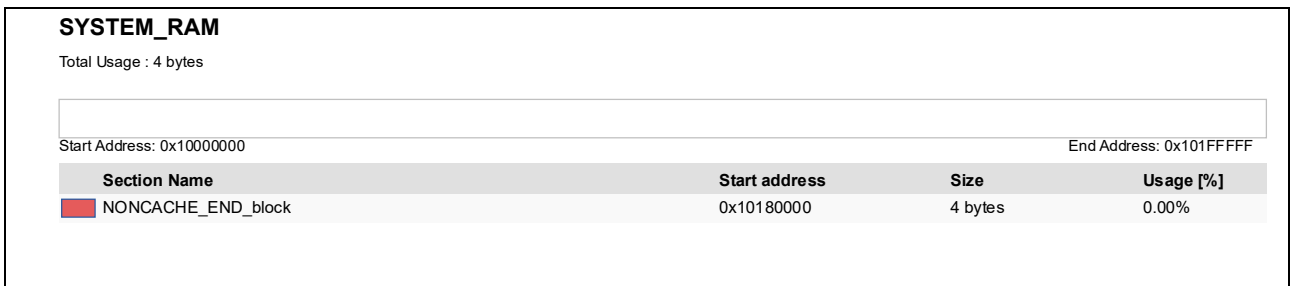
Figure 8.74. SYSTEM_RAM footprint of the RZ/T2H, N2H (CA55_dual) Primary project (EWARM)
