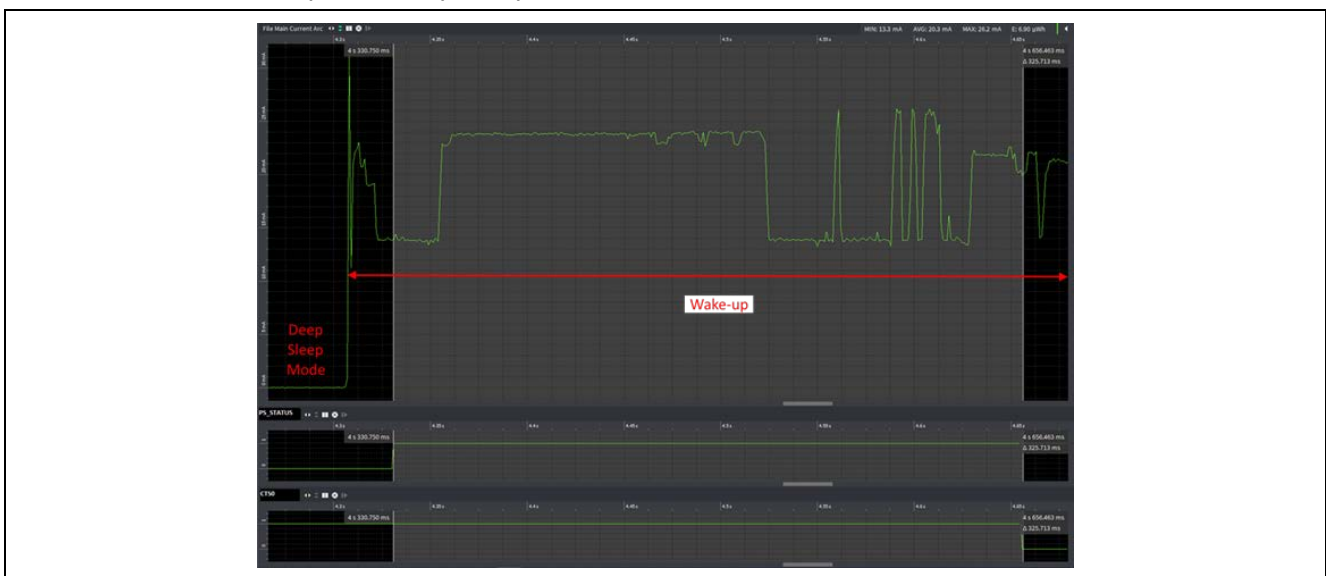
Figure 6. Modem Wakes up from Deep Sleep Mode
