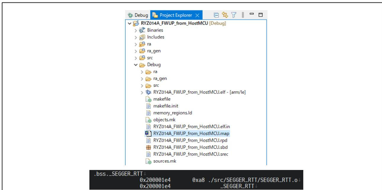
図 3-7 RTT Control Block Address
