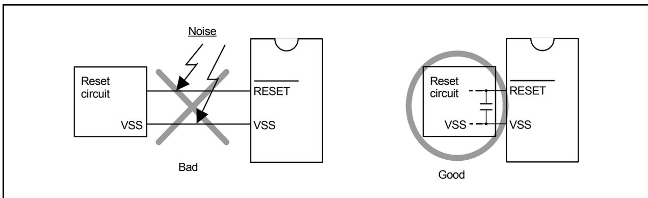
Figure 1.1 Wiring for the  $\overline{\text{RESET}}$  Pin
