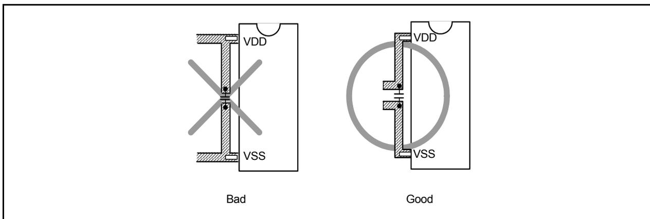
Figure 1.3 Bypass Capacitor Across the VSS Line and VDD Line
