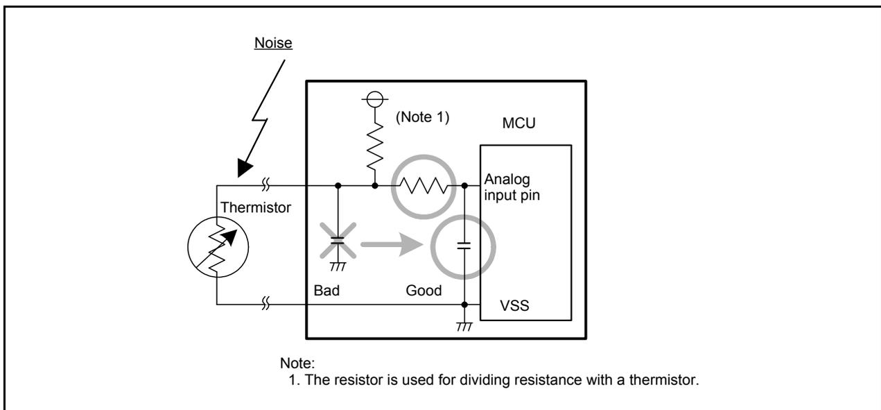
Figure 1.4 Analog Signal Line, a Resistor, and a Capacitor
