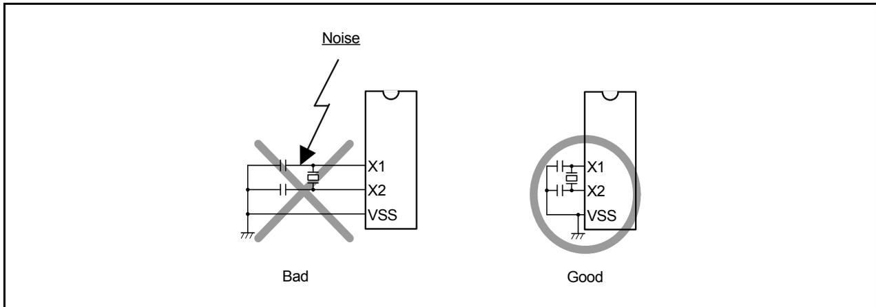
**Figure 1.2** Wiring for Clock Input/Output Pins
