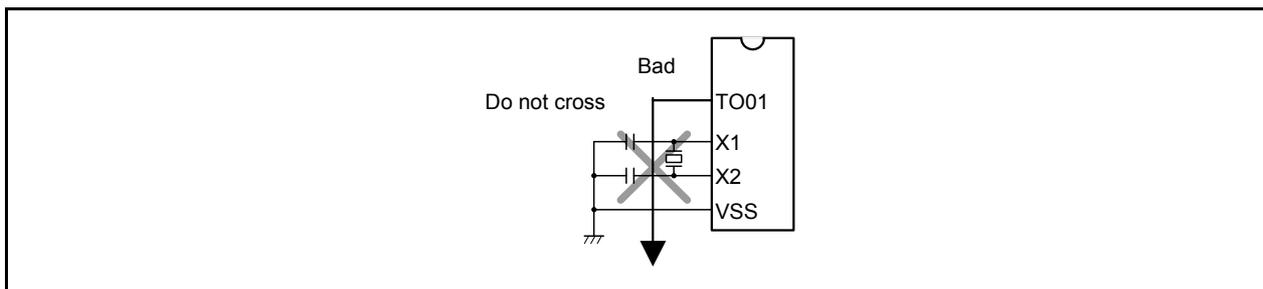
Figure 1.6 Wiring of Signal Lines Where Potential Levels Change Frequently
