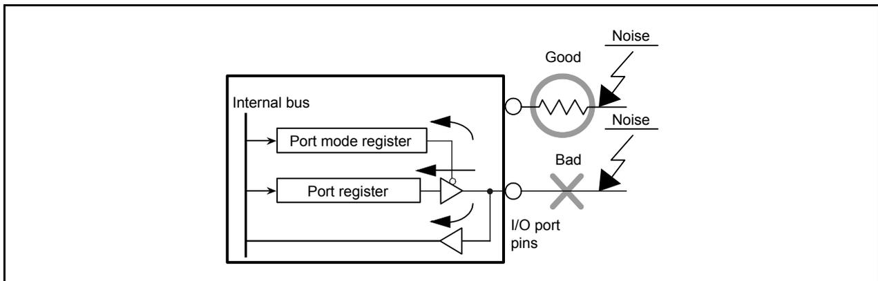
Figure 1.7 Setup for I/O Ports
