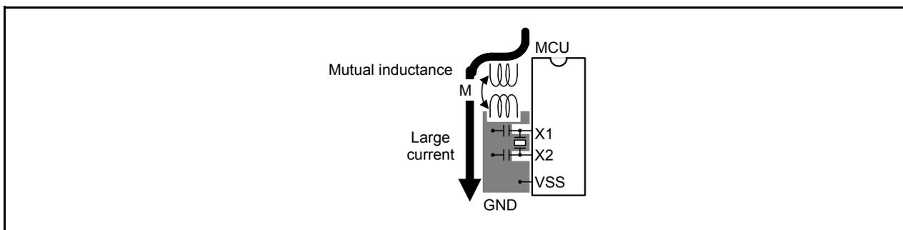
Figure 1.5 Wiring of a Large Current Signal Line
