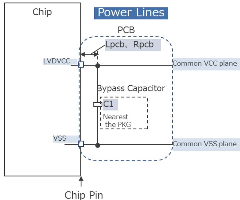
Figure 2.1 Connection Example of Power Wiring
