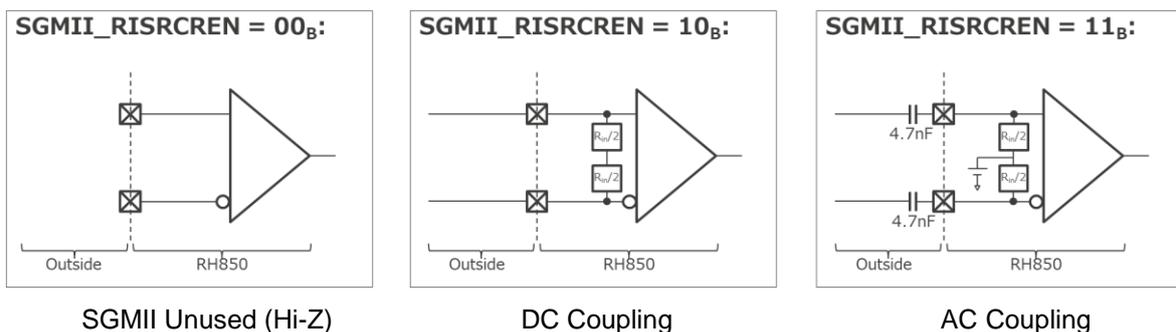
Figure 3.5 Setting Example of Rx pin state
