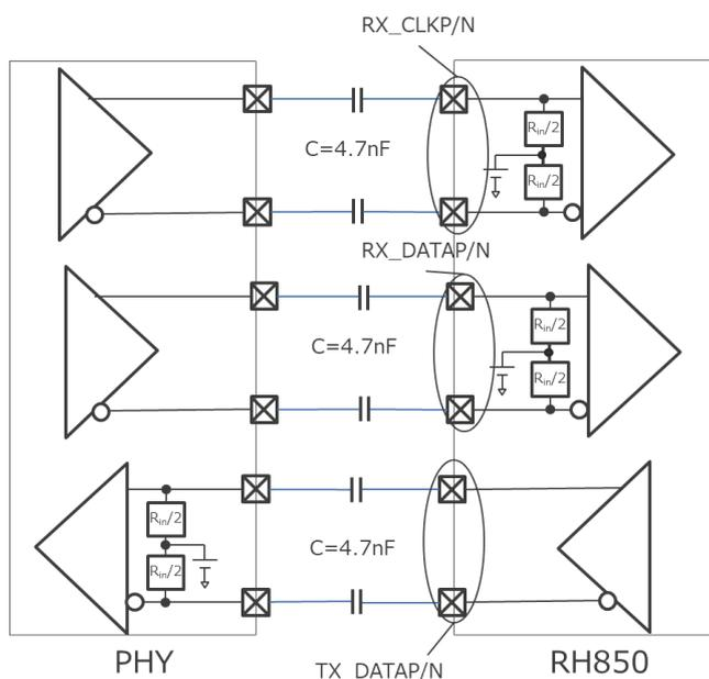
Figure 3.4 Connection Example with AC Coupling (U2A-EVA)
