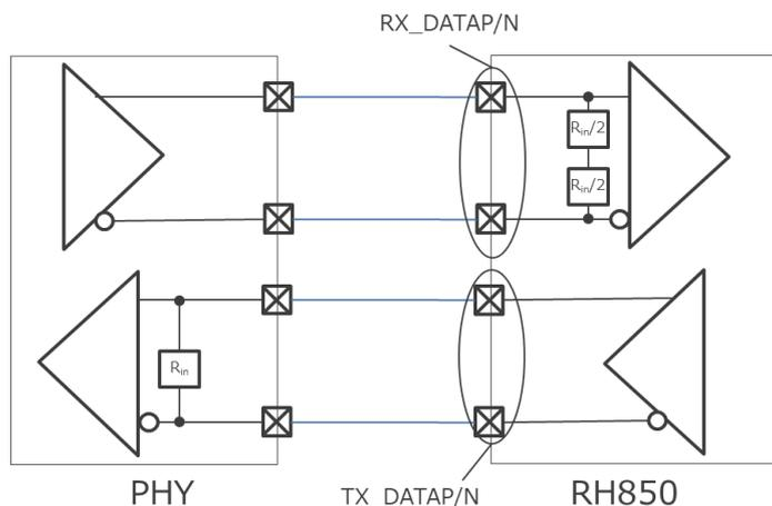
Figure 3.1 Connection Example with DC Coupling
