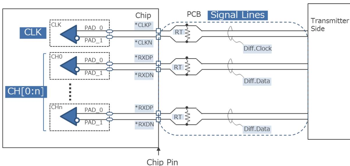
Figure 1.1 Connection Example of LVDS
