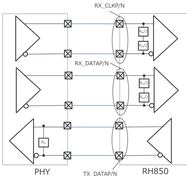
Figure 3.3 Connection Example with DC Coupling (U2A-EVA)
