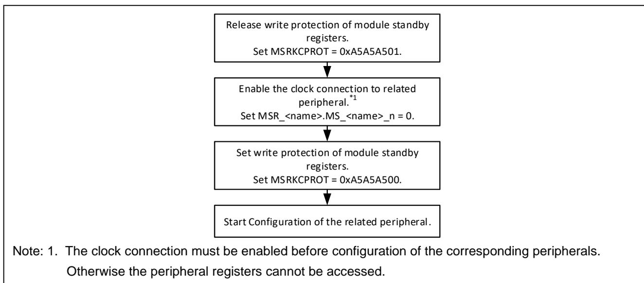
**Figure 7-2 Setting Procedure of Peripherals in Sample SW**
