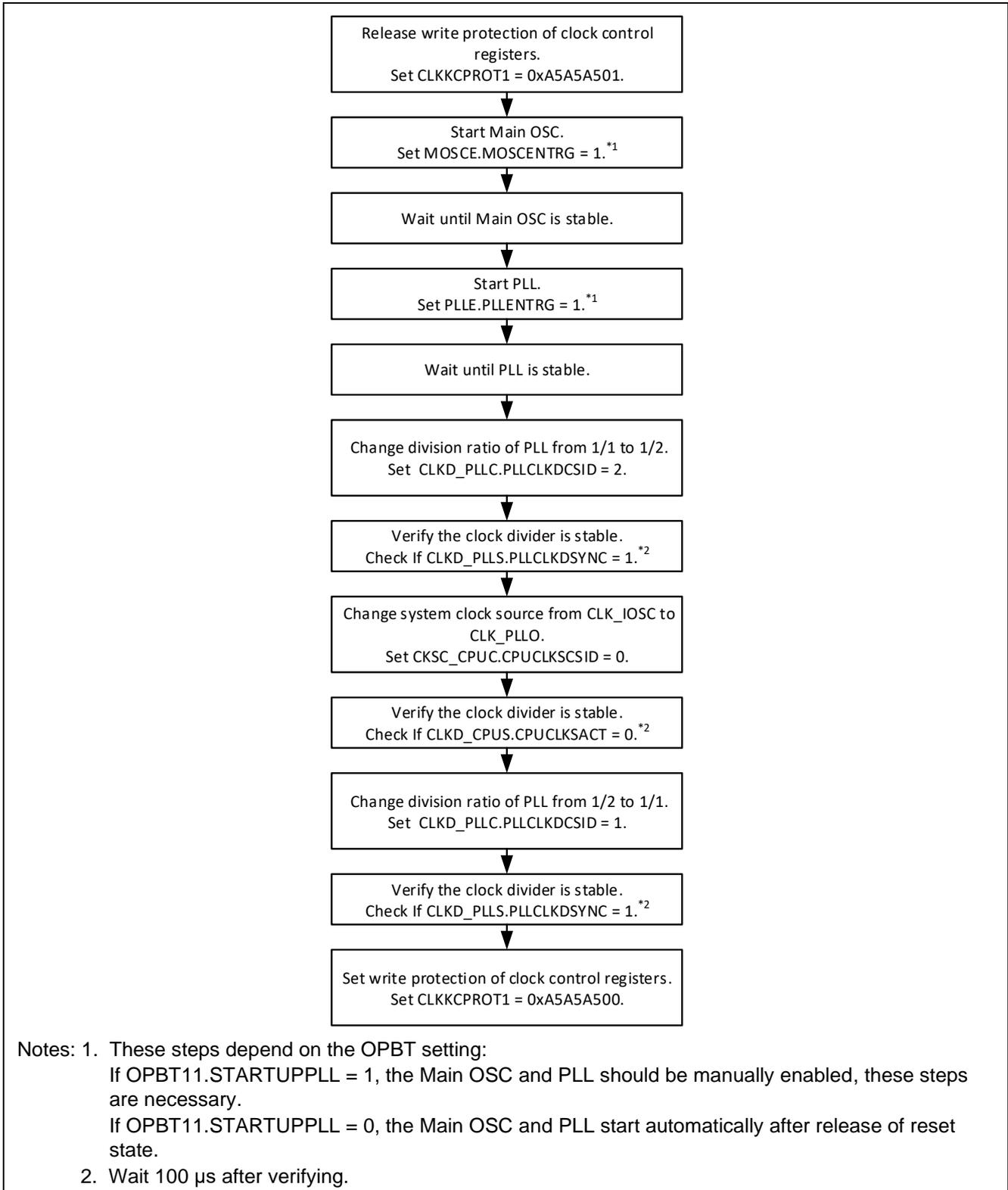
Figure 7-1 Setting Procedure of System Clock in Sample SW
