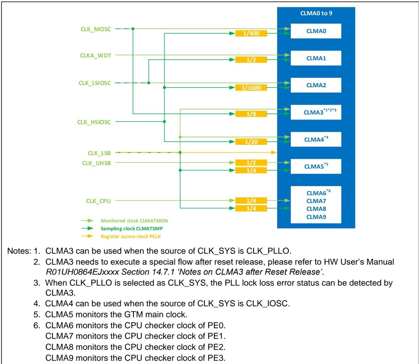
Figure 4-3 Clock Supply of Clock Monitor (CLMA)
