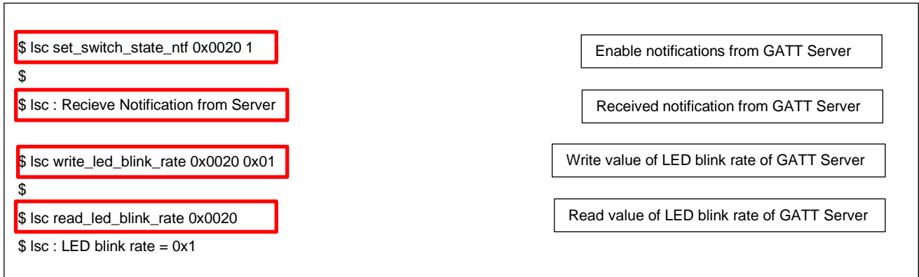
Figure 20. LED switch service commands and responses
