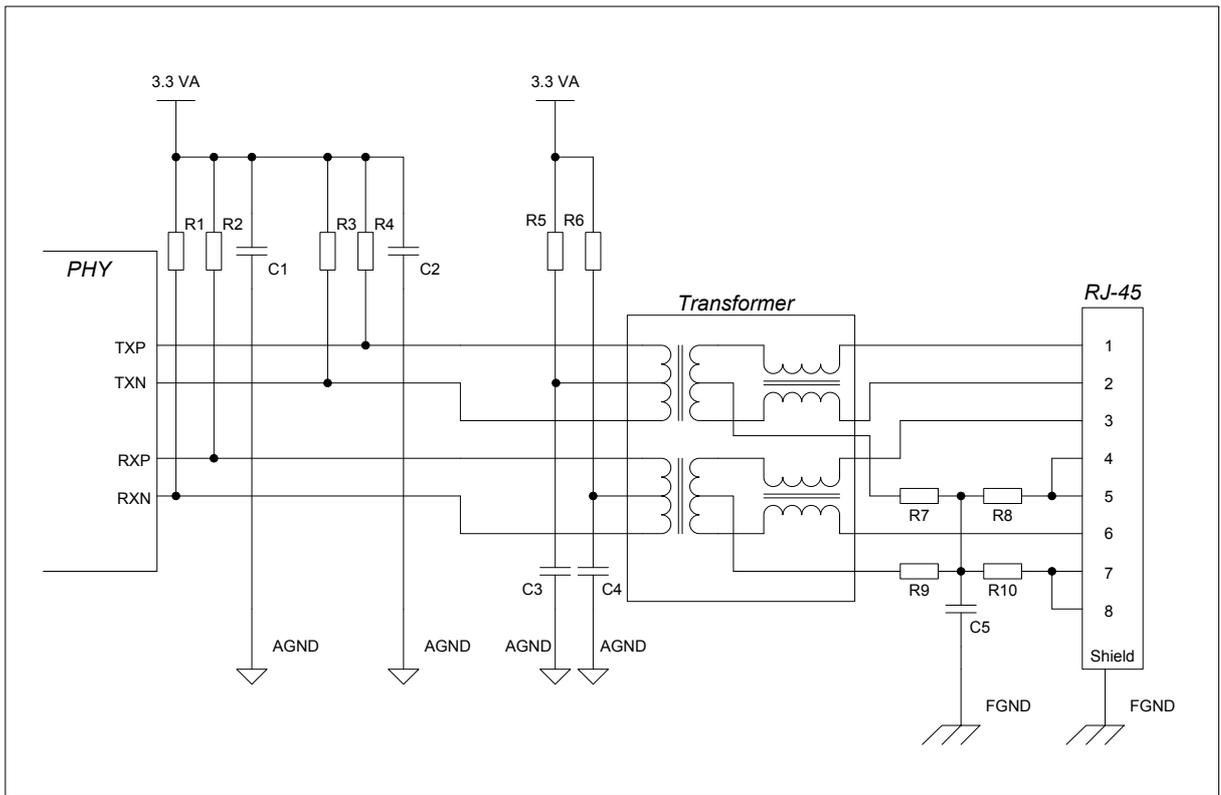
Figure 3-5 Schematics for twisted pair interface circuit with integrated magnetics
