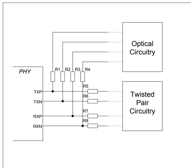
Figure 3-10 Layout Example parallel twisted pair and optical preparation
