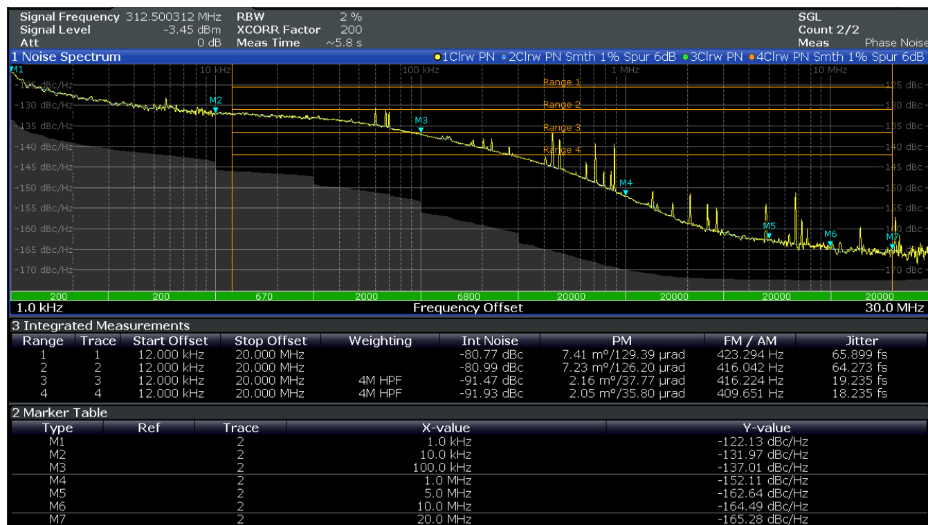
Figure 2. Phase Noise Plot for a 312.5MHz Output from an RC32312 FC3 Device Operating in Jitter Attenuator Mode, using a 49.152MHz Crystal along with an APLL VCO Frequency of 10GHz, and a 25MHz + 1ppm Reference Input, measured using a Rohde & Schwarz FSWP; RMS Jitter also displayed
