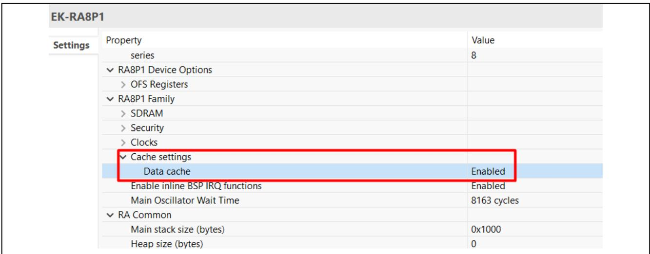
Figure 37. Example of CM85 Data Cache (D-Cache) Enabled
