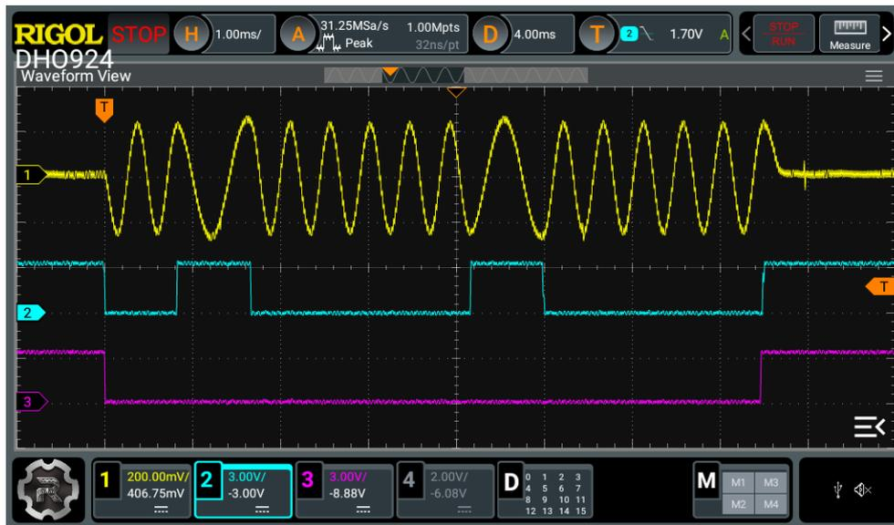
Figure 7. Sending Data to the Current Loop (Data is 0x11)
