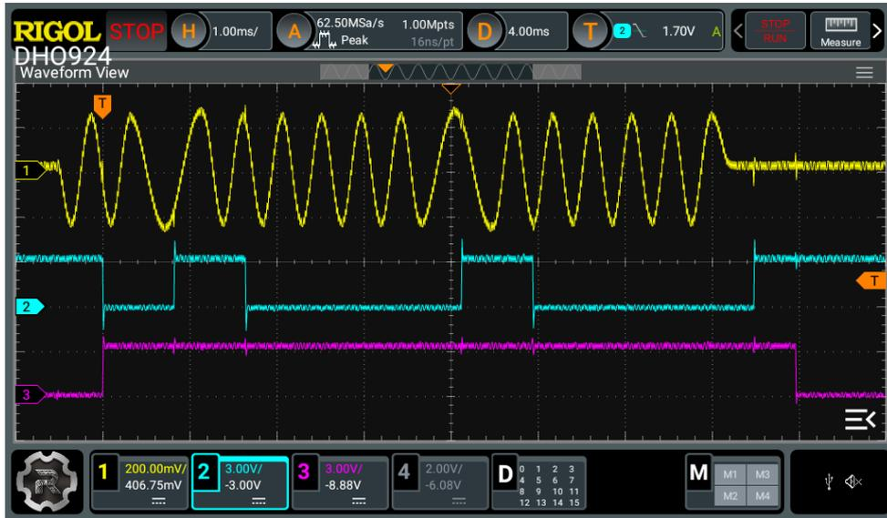
Figure 8. Receiving Data from the Current Loop
