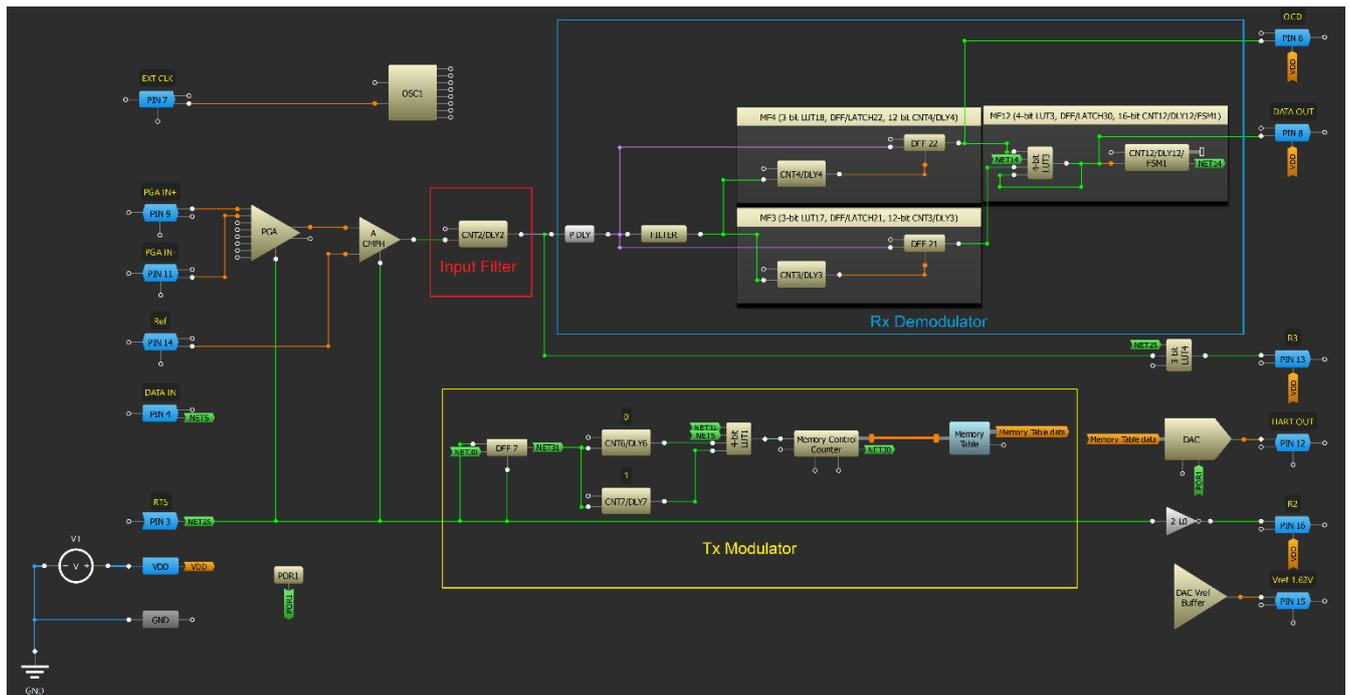
Figure 6. Go Configure Schematic of HART Modem
