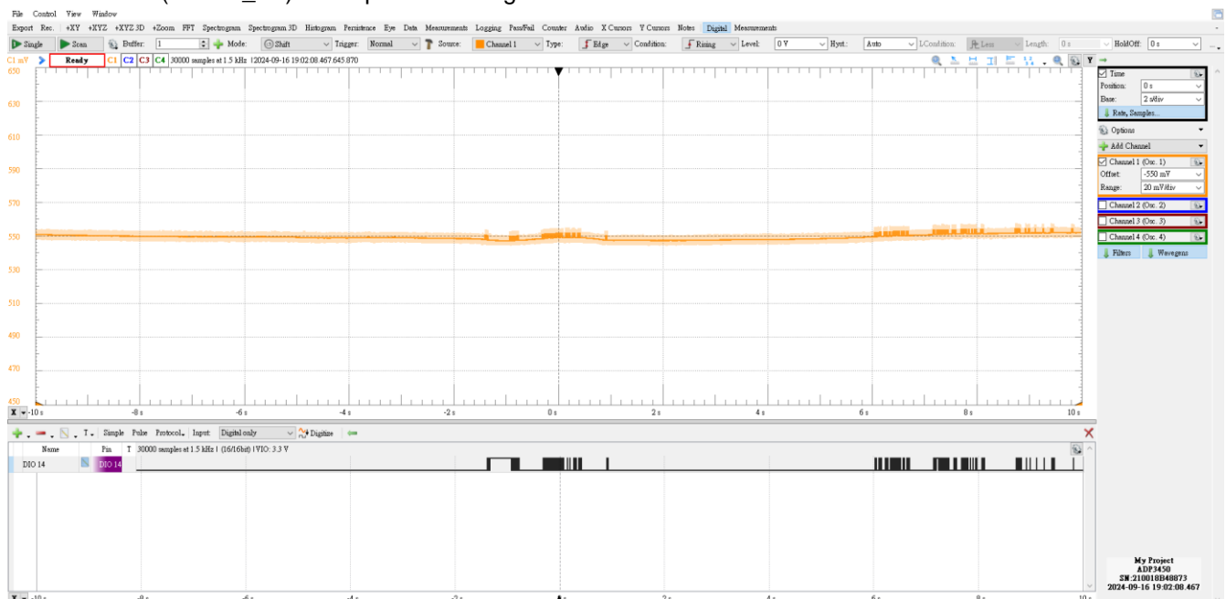
Figure 11. PIR signal measurement at 2 meters
