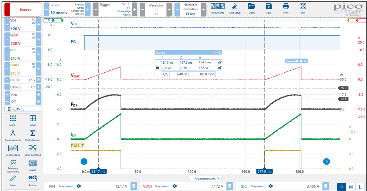
Figure 9: 12.5 W SOA operating waveform for SLG59H1132V for V_{IN} = 12 V, ON = Low → High, C_{SLEW} = 150 nF, R_{SET} = 14 k \Omega , C_{LOAD} = 10 \mu F, R_{LOAD} = 2 \Omega
