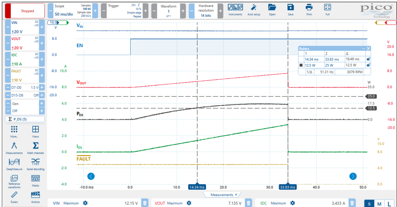
Figure 10: SLG59H1132V 12.5 W SOA operating waveform for V_{IN} = 12 V, ON = Low → High, C_{SLEW} = 150 nF, R_{SET} = 14 k \Omega , C_{LOAD} = 10 \mu F, R_{LOAD} = 2 \Omega (Extended view)
