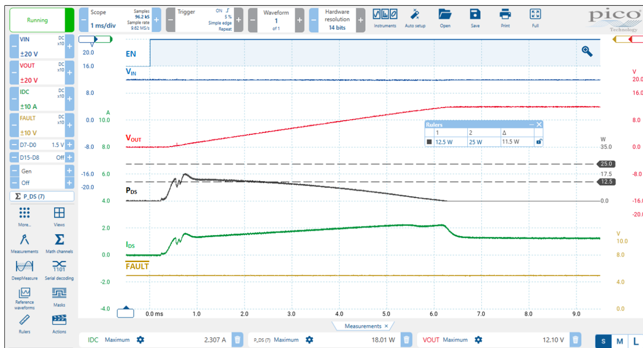
Figure 21. Turn-on operation waveform for V_{IN} = 12 \text{ V} , C_{SLEW} = 16 \text{ nF} , R_{SET} = 14 \text{ k}\Omega , C_{LOAD} = 600 \text{ }\mu\text{F} , R_{LOAD} = 10 \text{ }\Omega
