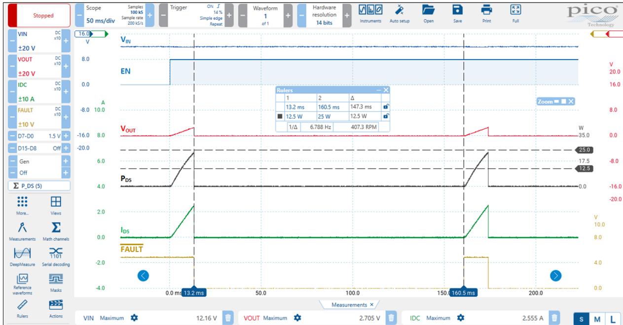
Figure 7: SLG59H1132V 25 W SOA operation waveform for V_{IN} = 12\text{ V} , ON = Low \rightarrow High, C_{SLEW} = 150\text{ nF} , R_{SET} = 14\text{ k}\Omega , C_{LOAD} = 10\text{ }\mu\text{F} , R_{LOAD} = 1\text{ }\Omega
