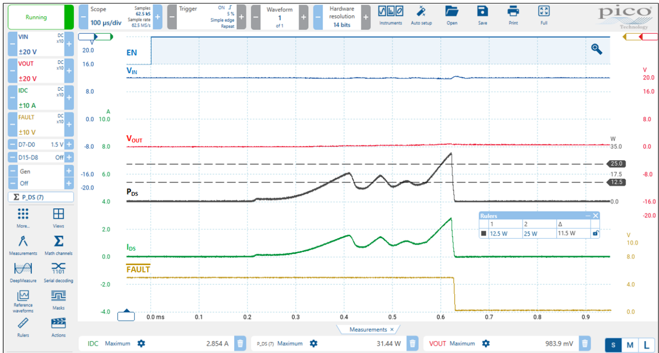
Figure 20. Turn-on operation waveform for V_{IN} = 12\text{ V} , C_{SLEW} = 10\text{ nF} , R_{SET} = 14\text{ k}\Omega , C_{LOAD} = 600\ \mu\text{F} , R_{LOAD} = 10\ \Omega
