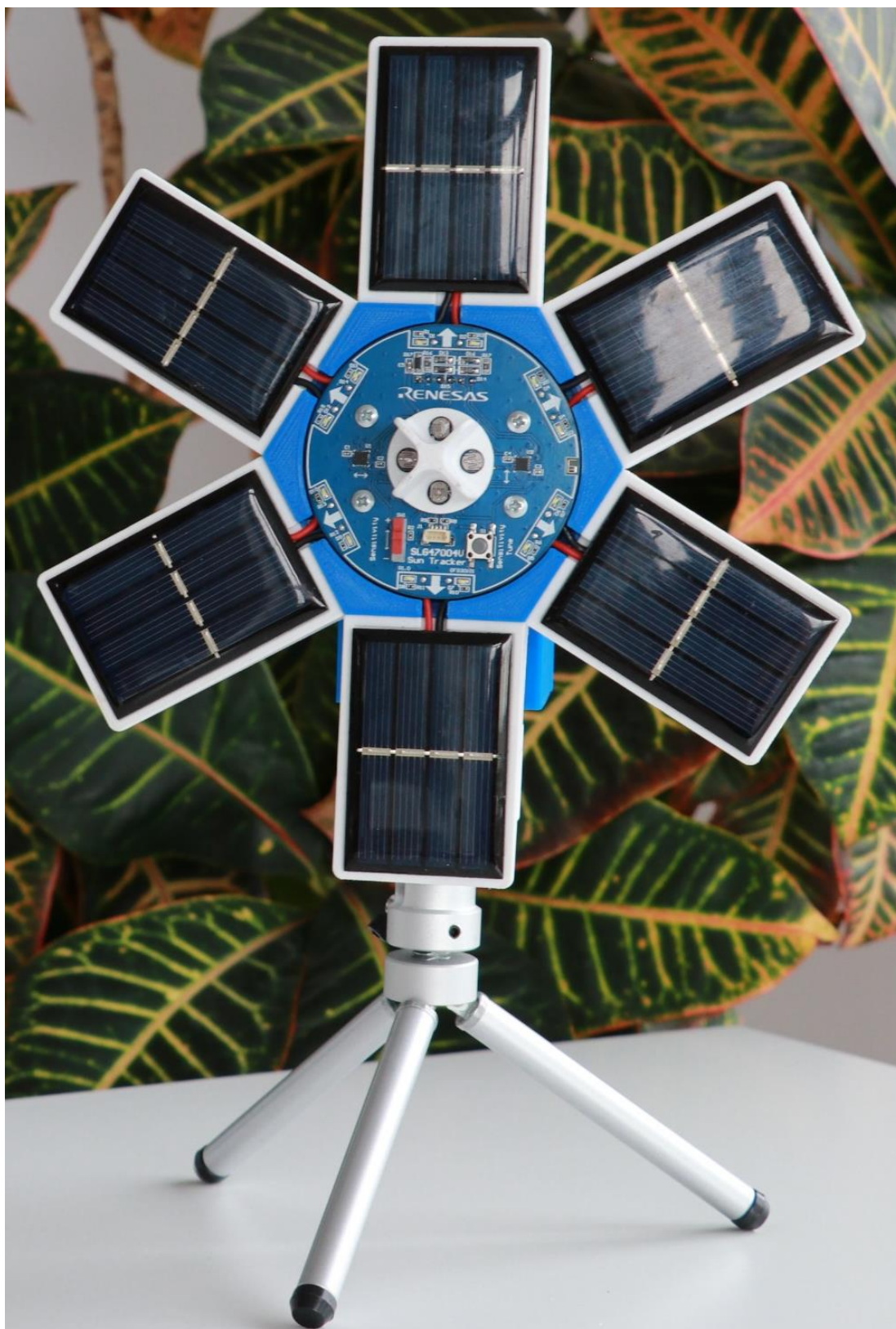
Figure 8. Front View of the Finished Model of the Sun Tracker
