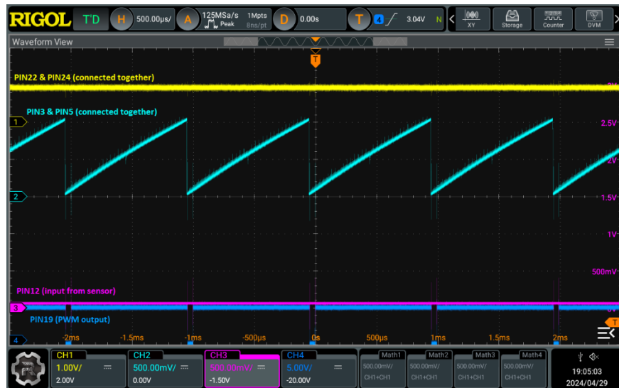
Figure 17: Operation of the PWM generation circuit. Duty cycle is ~95%
