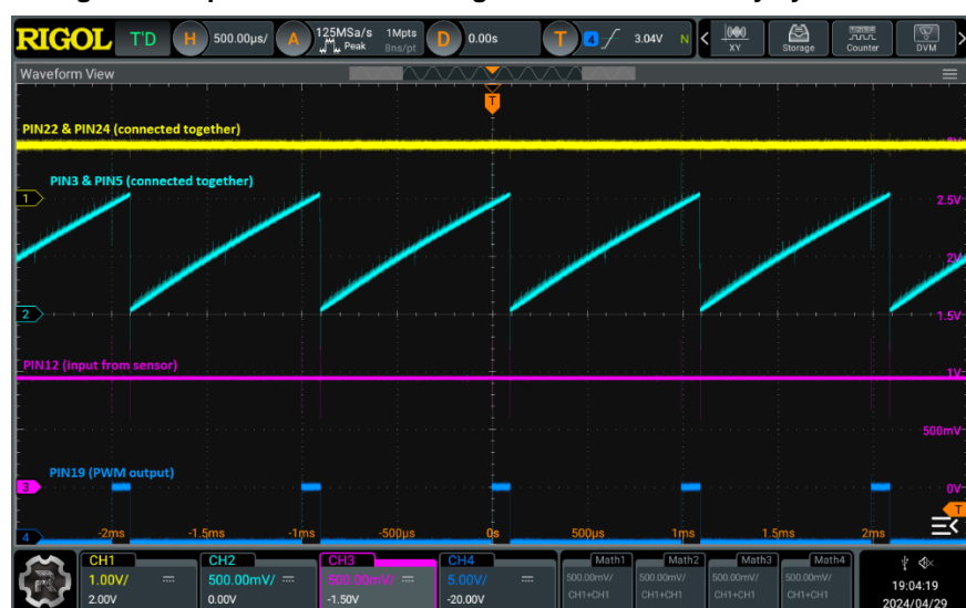
Figure 15: Operation of the PWM generation circuit. Duty cycle is ~10%
