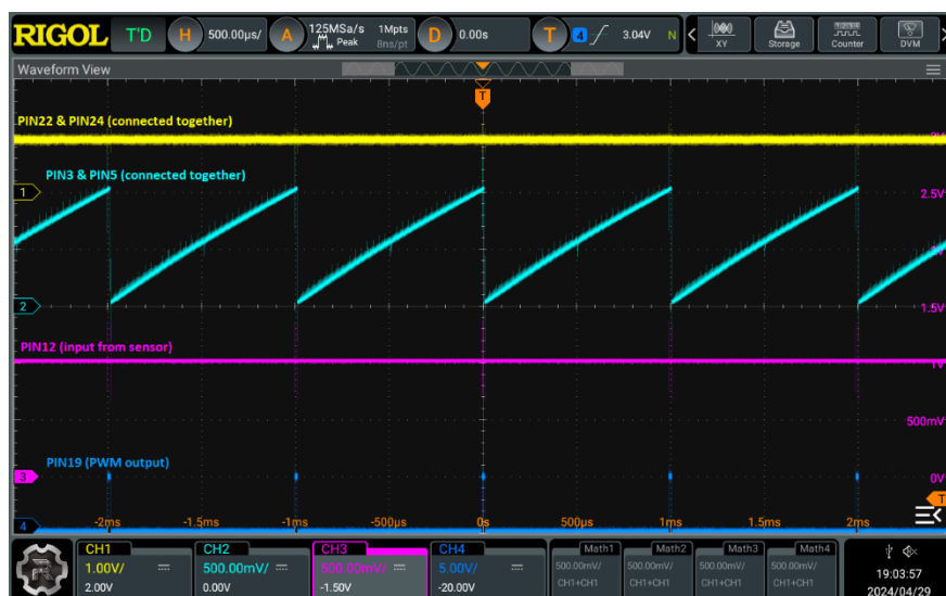
Figure 14: Operation of the PWM generation circuit. Duty cycle is ~1%
