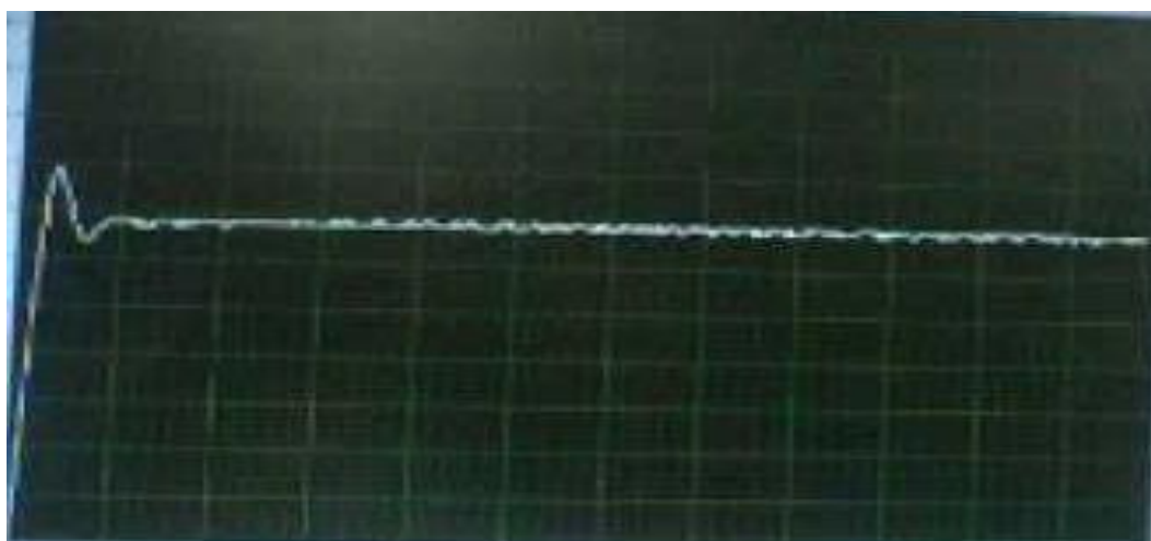
Figure 24: Oscilloscope Screenshot of the System Reaching a Stable System Response
