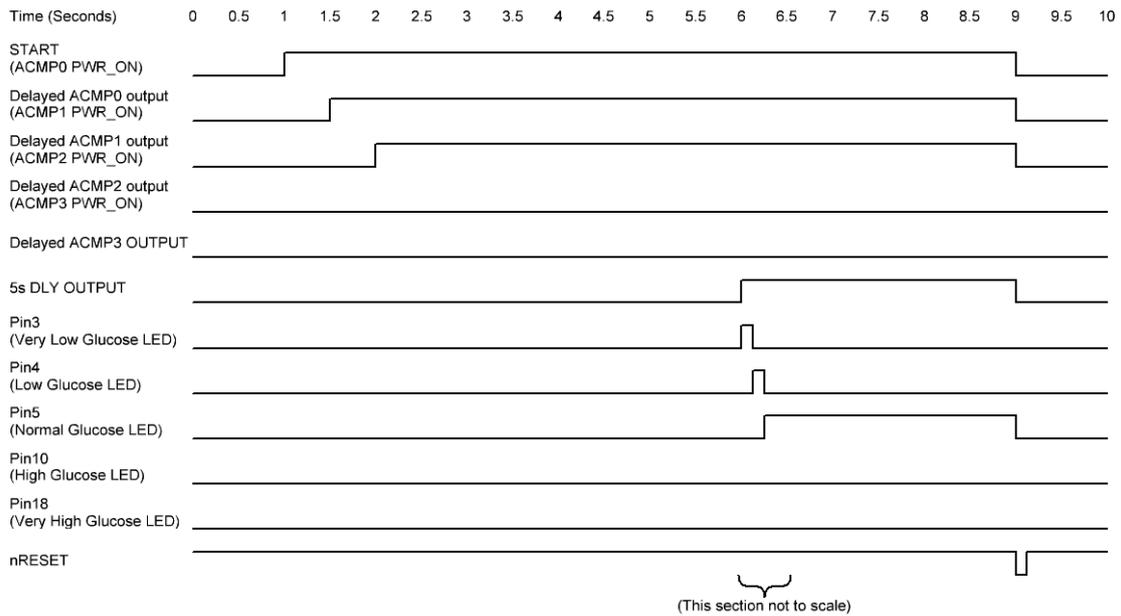
Figure 4: System signals when 300mv < ANALOG\_IN < 350mv
