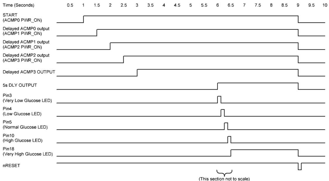
Figure 5: System Signals when ANALOG\_IN > 400 mv
