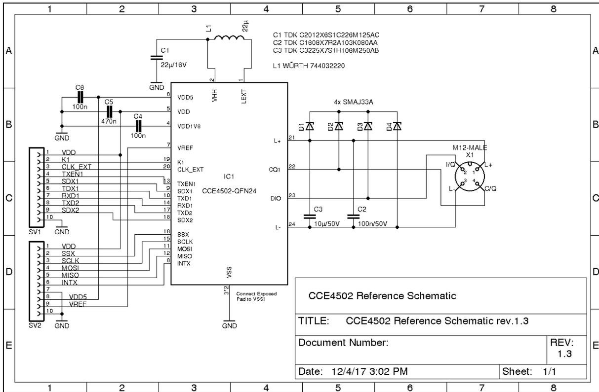
Figure 8: CCE4502 IO-Link Device Reference Schematic
