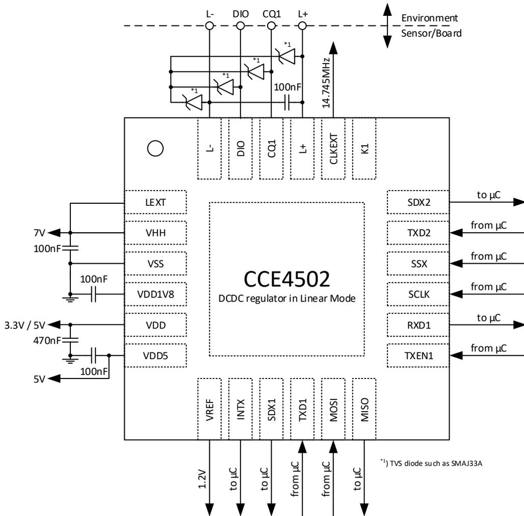
Figure 4: Application schematic with DC/DC in Linear Mode
