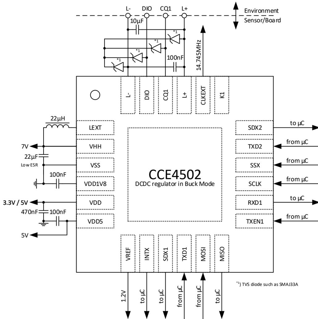
Figure 3: Application schematic with DC/DC in Buck Mode
