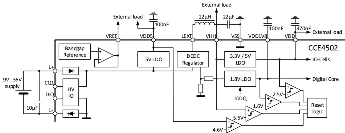
**Figure 2: CCE4502 power supply block diagram**
