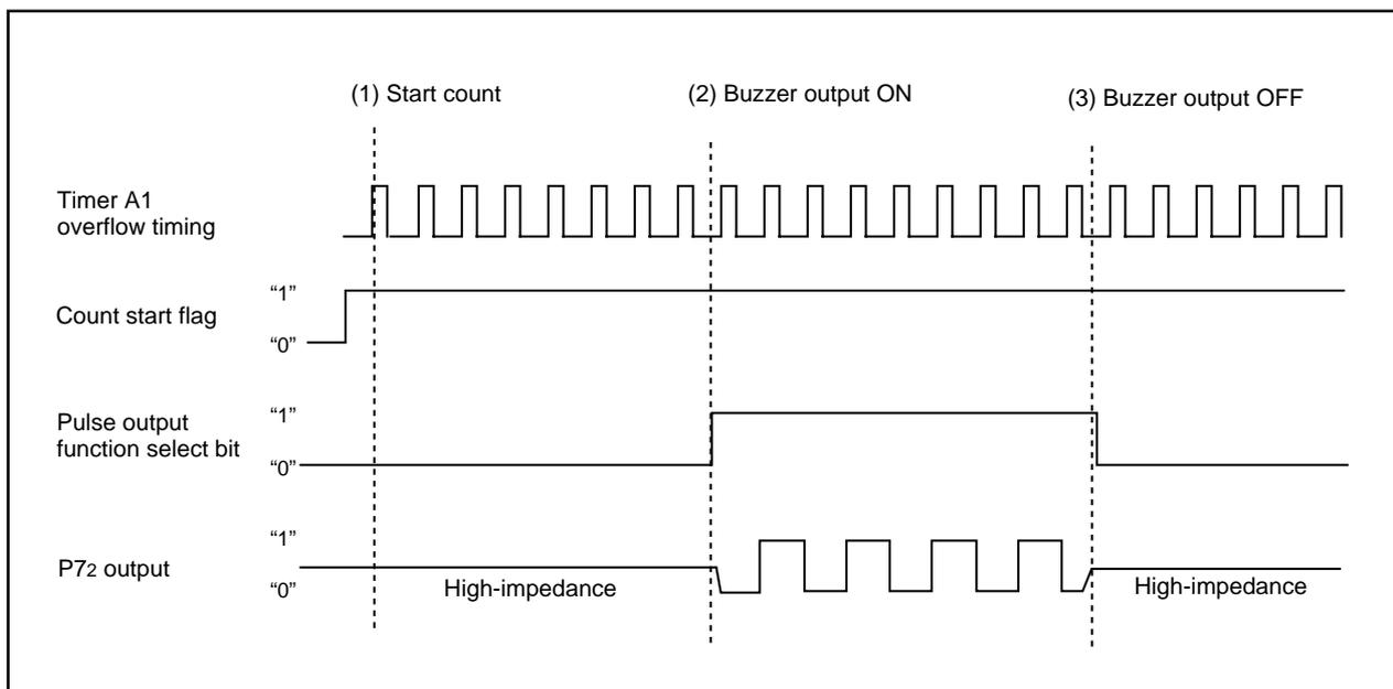
Figure 1. Operation timing of buzzer output
