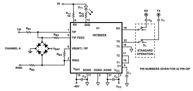
Schematic Diagram for Standard Operation
