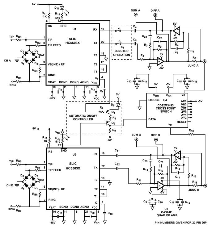
FIGURE 6. APPLICATION SCHEMATIC FOR JUNCTOR OPERATION
