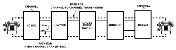
FIGURE 5. INTRA-CHANNEL AND CHANNEL-TO-CHANNEL PATHS THROUGH THE SYSTEM
