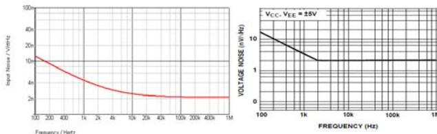
FIGURE 13. INPUT NOISE VOLTAGE VERSUS FREQUENCY FOR MACRO MODEL (LEFT) AND DEVICE DATA SHEET (RIGHT)
