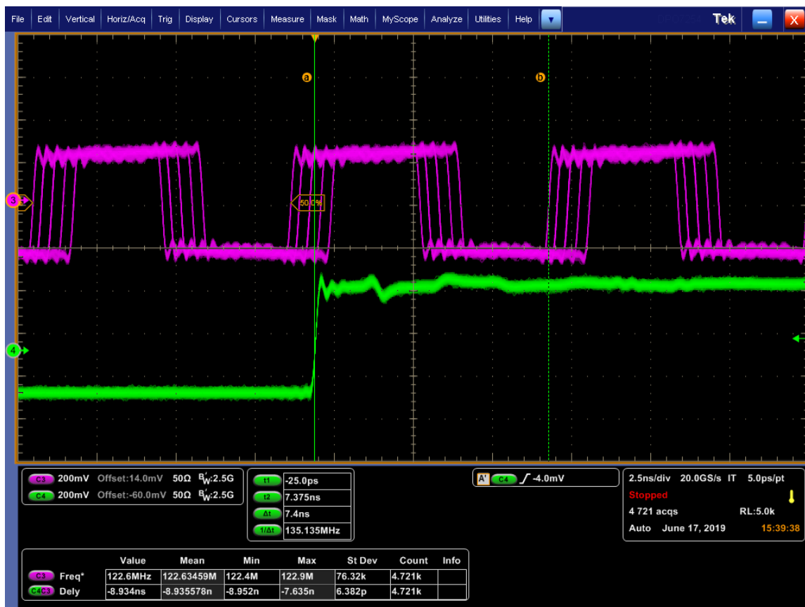
Figure 3. Result of Adjusting Individual Sysref Phase Delay
