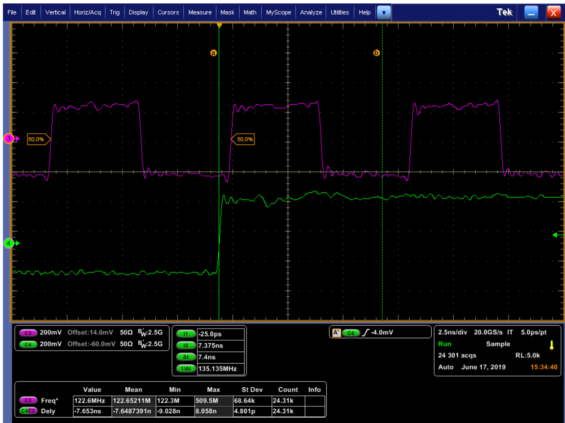
Figure 2. Sysref to QCLK Delay after Updating Sysref Global Phase Delay
