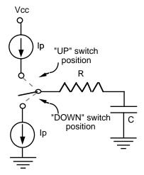
Figure 4. Charge Pump & Loop Filter configuration
