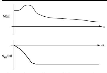
Figure 6. Example of Bode magnitude and phase plots
