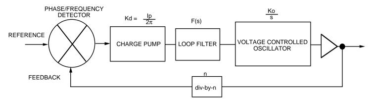
Figure 1. Phase-Lock Loop
