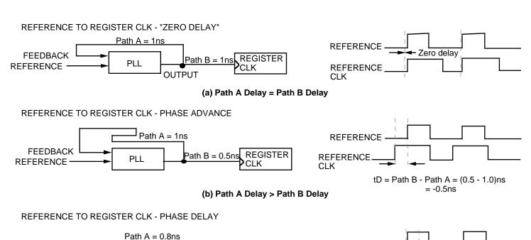
Figure 7. Delay Compensation using PLLs
