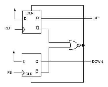
Figure 2. Phase Frequency Detector
