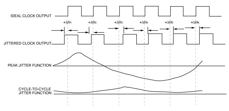
Figure 9. Output jitter
