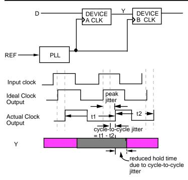
Figure 10 Peak vs Cycle-to-cycle jitter
