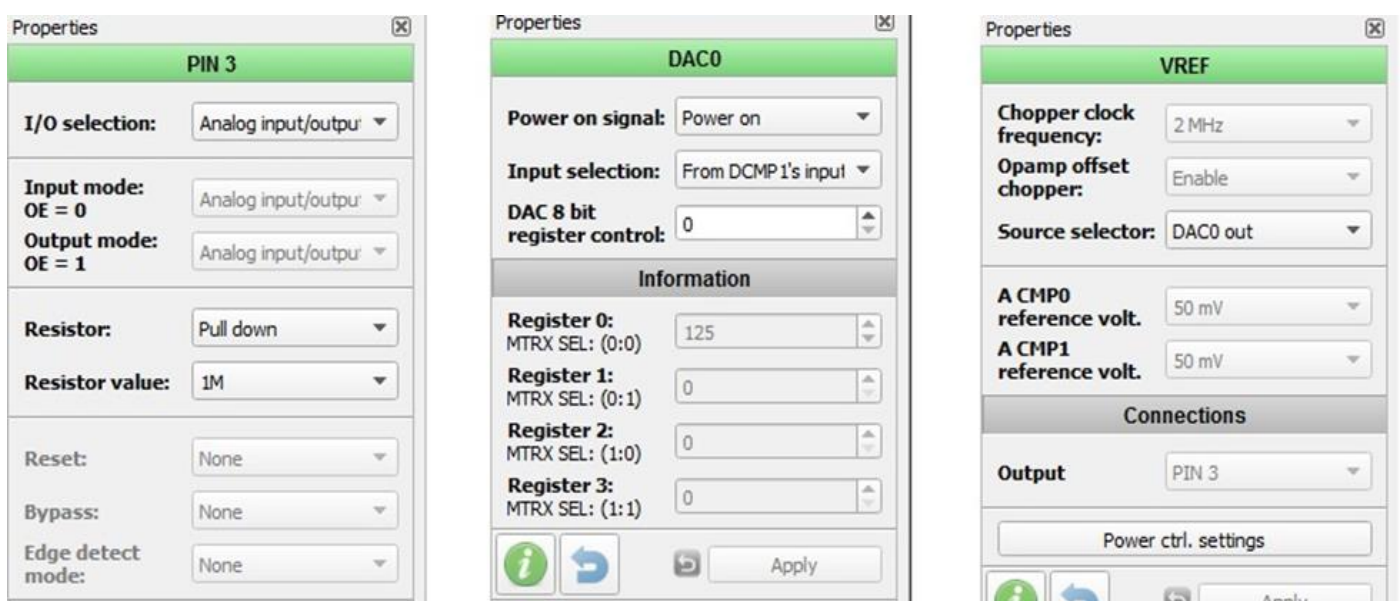
Figure 5. Pin 3, DAC0 and VREF settings
