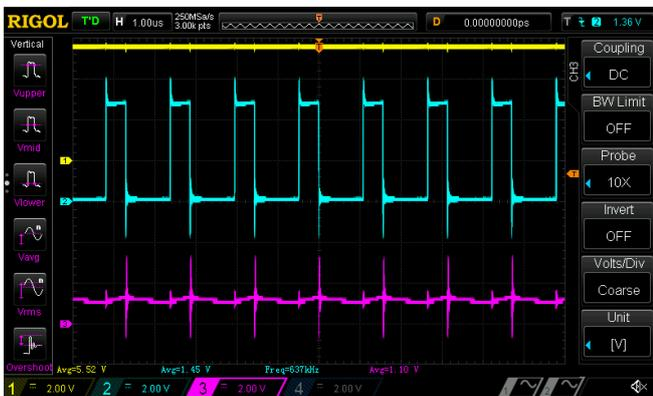
**Figure 3. Device functionality then SPI code 255 at VDD 5.5V**
